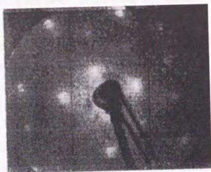
Fig. 7-1-1: A LEED pattern of \text{SnSe}_2 (2ML thickness) / 1\text{T-TaS}_2 . Acceleration voltage is 115eV.
