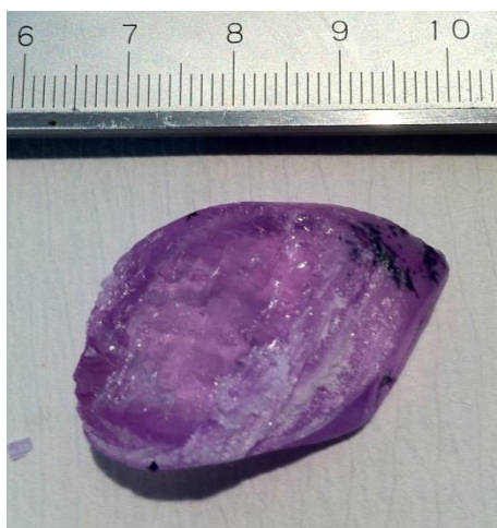
a. A roughly cut crystal. The surface is a-c plane.
