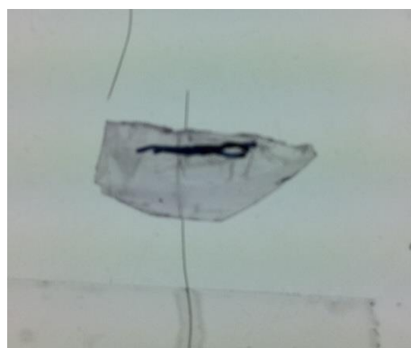
d. Under a polarizer on horizontal direction, the hair under the crystal was shift. The shift direction indicates the c-axis.
