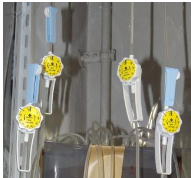
Figure 3-6- Medical drip used as a rainfall simulator
