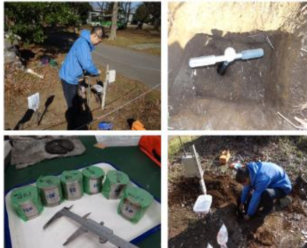
Figure 2-3-Penetration test, Chiba soil sample were collected, at IIS, Nishi Chiba
