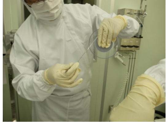
Figure 5.25: The indium ribbon for the sealing.
