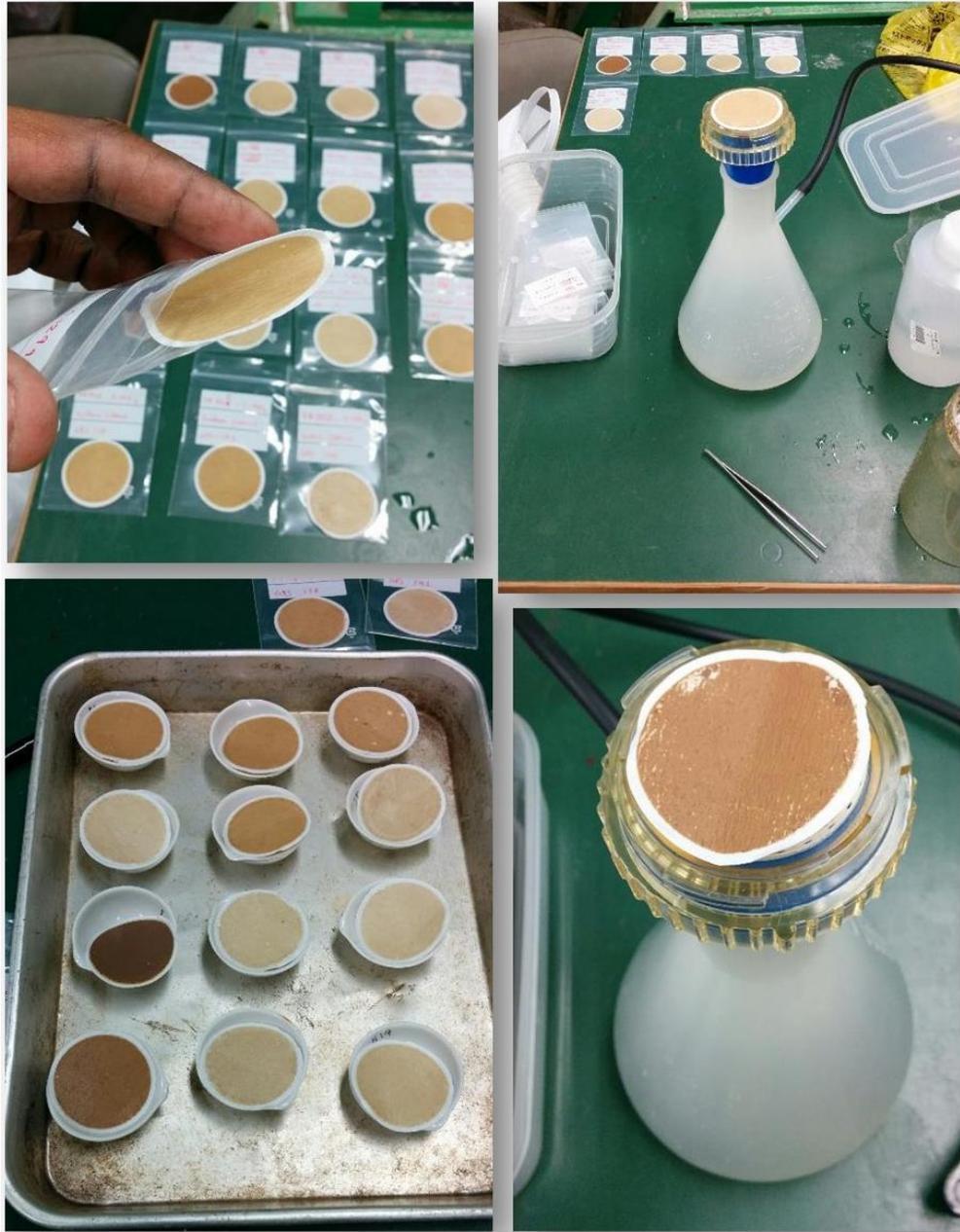
Figure 3.12 Sample preparation for weight measurements
