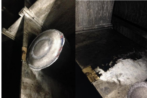
Figure I-8 Black color in the wind tunnel after test.
