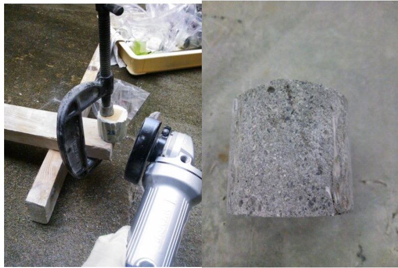
Figure 3-24 Removing epoxy coating from mortar specimen.
