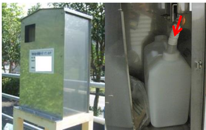
Figure 3-26 PWRI airborne chloride capture equipment.
