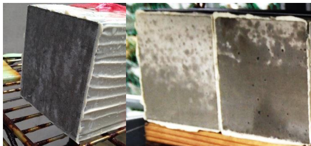
Figure 4-53 Concrete specimen under light rainfall (1-3 mm/hr).
