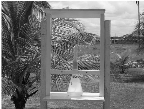
Figure 4-87 Wet candle equipment set [24]
