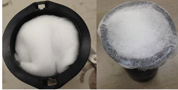
Figure 4-19 Cotton and gauze specimen for measuring amount of airborne chloride.
