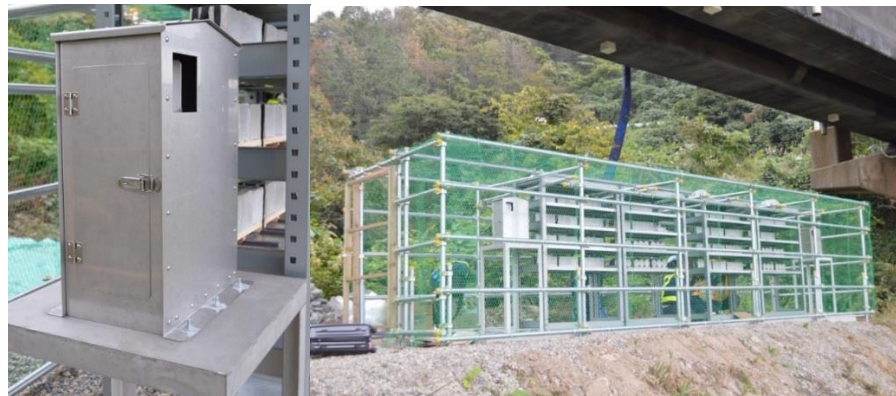
Figure 4-74 Airborne chloride capture tank [19].
