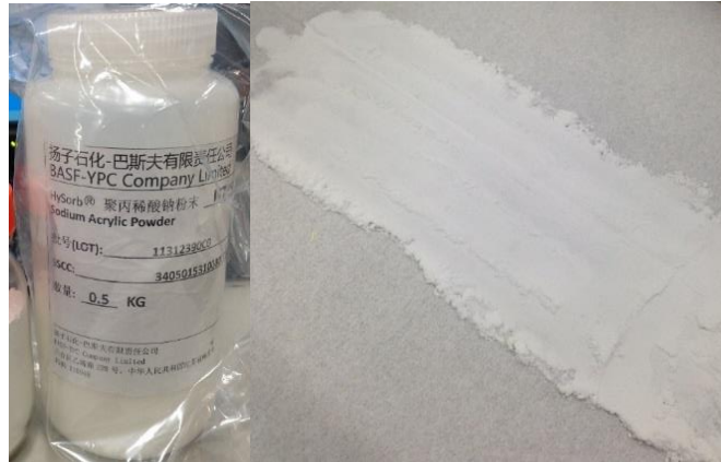
Figure I-22 Super absorbent polymer. (BASF-YPC, Sodium acrylic powder)
