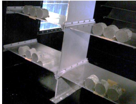
Figure 2-27 Mortar specimen installation position.
