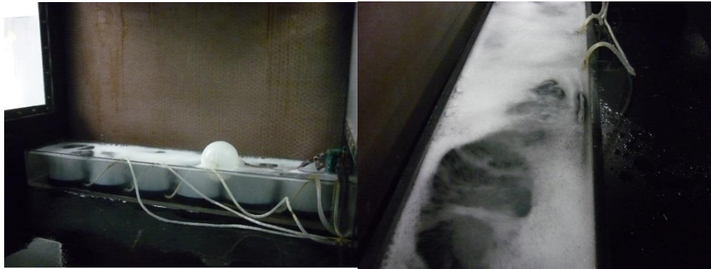
Figure 2-22 Salt bath and bubble generator inside the wind tunnel [29].
