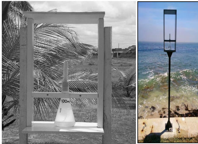
Figure 2-7 Example of wet candle device setup [15, 16].
