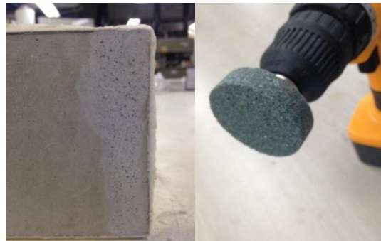
Figure 4-25 Surface grinding before submersion.
