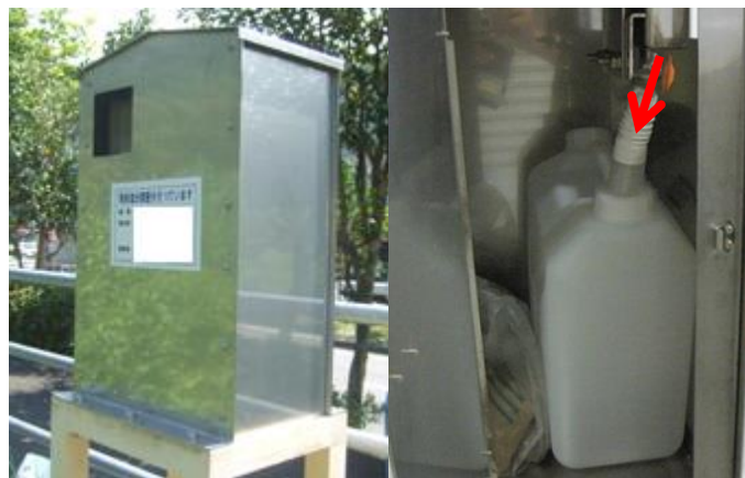
Figure 5-7 The PWRI airborne chloride capture equipment.
