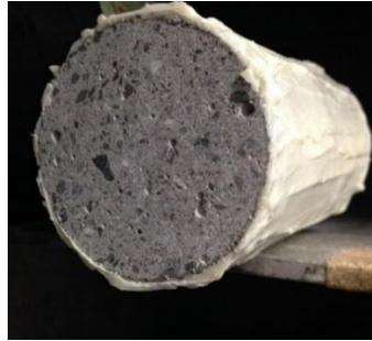
Figure 4-20 Specimen for water ingress test.
