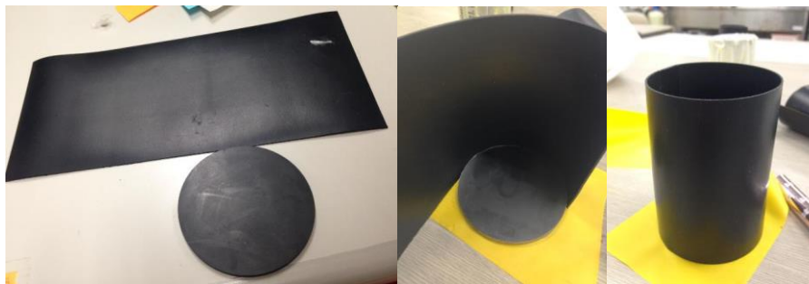
Figure I-18 Rubber mold size \text{Ø}7 cm x 10 cm.
