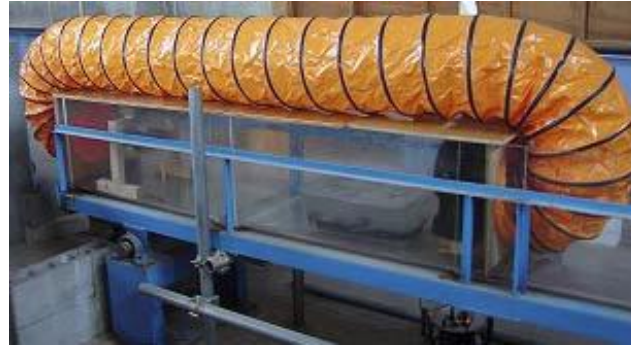
Figure 2-17 Wind tunnel prototype to simulate airborne chloride environmental conditions [23].
