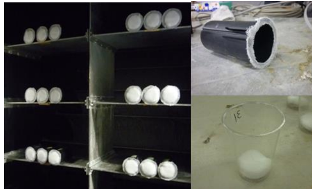
Figure 2-25 Gauze and cotton specimens.
