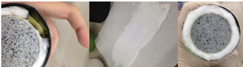
Figure I-19 Specimen filled with SAP materials.
