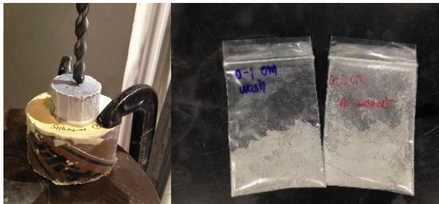
Figure 4-36 Drilling machine and powder specimen for titration.
