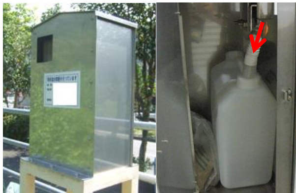
Figure 4-60 PWRI airborne chloride capture equipment.
