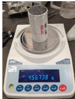
Figure 4-21 Measuring water ingress.
