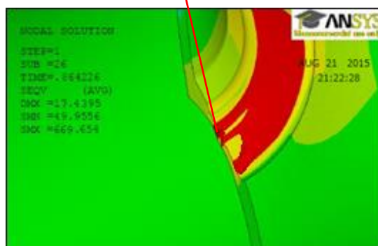
(d) All sectional cross reached the tensile stress (Internal pressure 19.1MPa)
