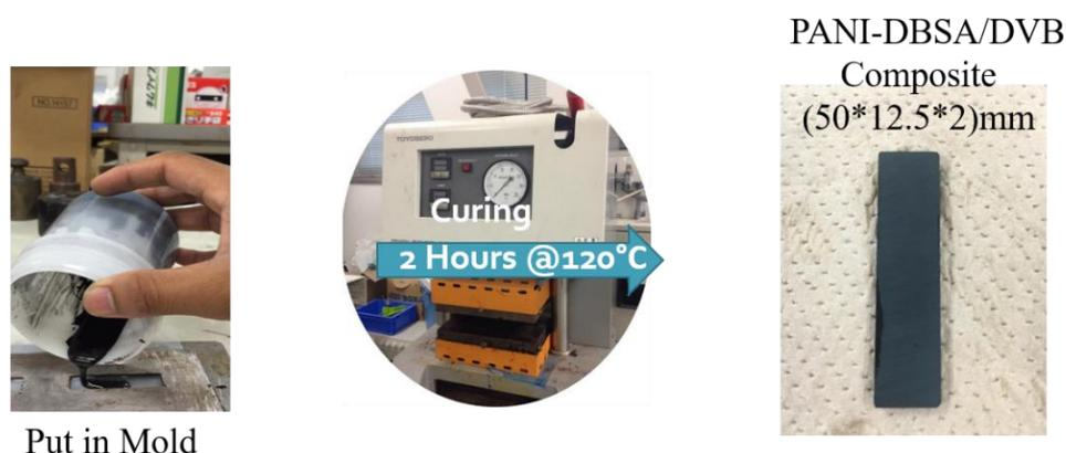
**Figure 4.1** Manufacturing of (PANI-DBSA)<sup>CM</sup>/DVB composite.
