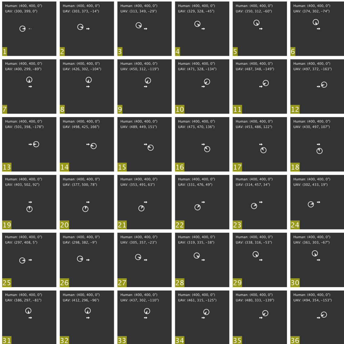
Figure 4.9: 2D simulation of circling behavior of a flying robot in Processing environment when the target is not moving. (See text for details.)
