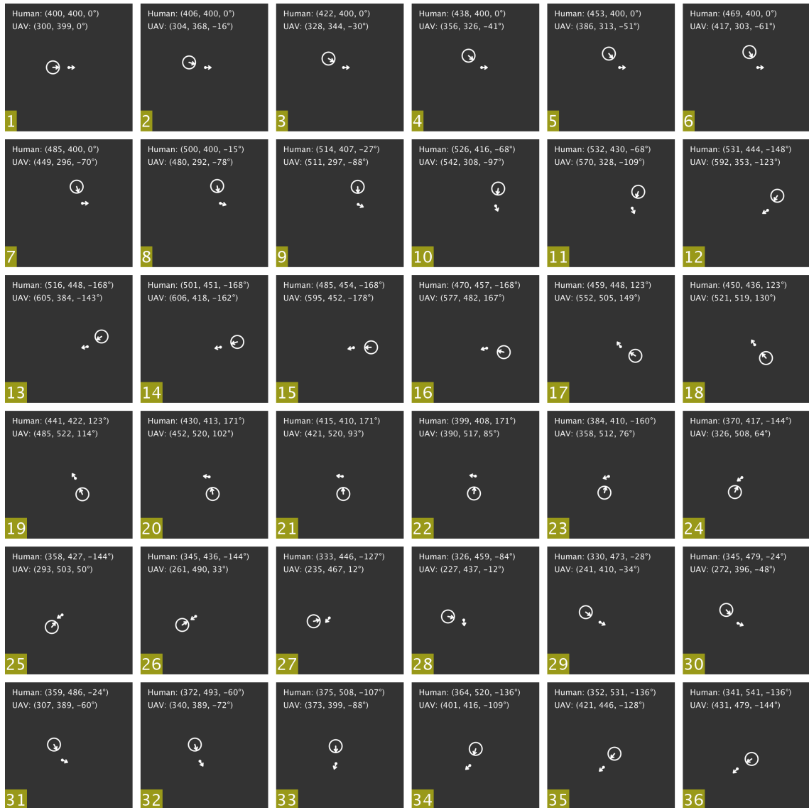
Figure 4.10: 2D simulation of circling behavior of a flying robot in Processing environment while the target is moving. (See text for details.)
