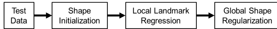
Figure 8.2: Framework overview. During the test, our system starts from shape initialization, followed by local landmark searching and global shape regularization.
