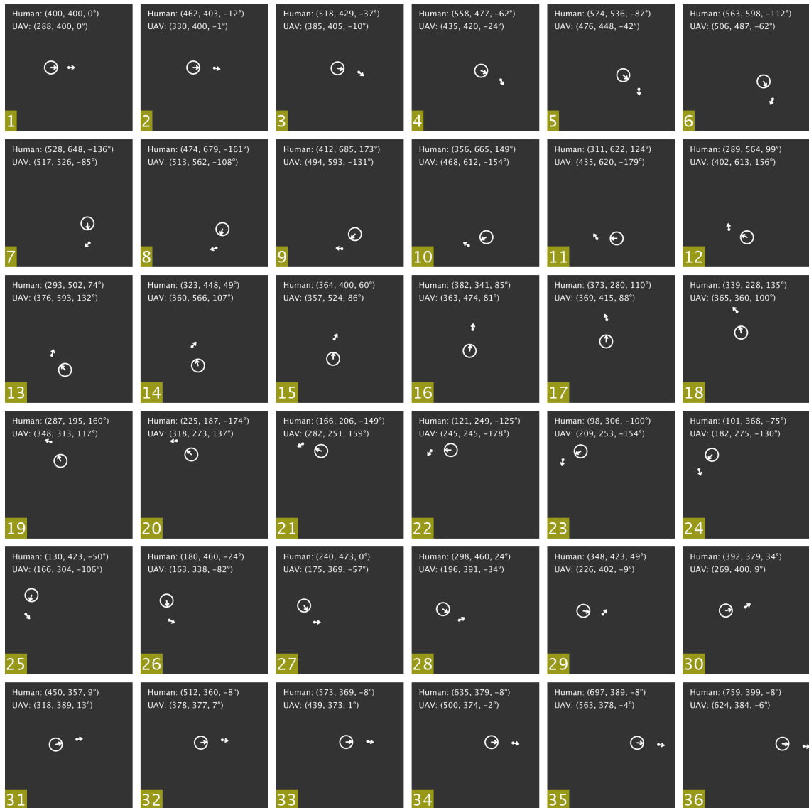
Figure 4.8: 2D simulation of following behavior of a flying robot in Processing environment. (See text for details.)
