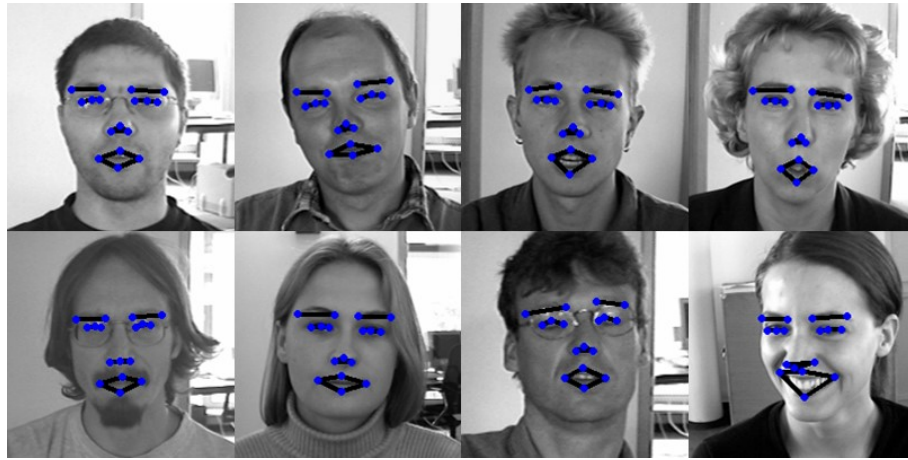
Figure 8.1: Face alignment, a process of locating facial feature points, has been used in various applications such as face recognition, facial expression recognition, and head pose estimation. Seventeen selected facial feature points are plotted on images taken from BioID Dataset [297].
