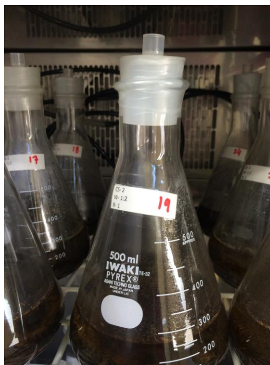
Figure 6.5 The experimental set-up without oxygen. Hole on the silicon stopper for gas sampling
