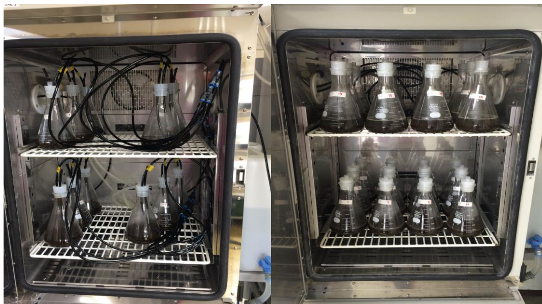
Figure 6.2 The experimental set-up i) with oxygen supply (left) and, ii) without oxygen supply (right)
