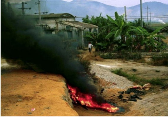
Open burning of wires and other parts to recover metals such as steel and Copper
