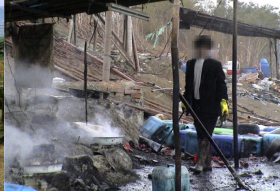
Gold recovering from waste PCBs using acid baths
