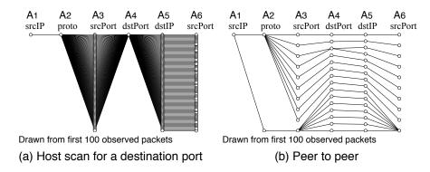
Figure 2.1: Examples of graphlets. Traffic from a single source host is represented as a graph connecting attributes such as proto, srcPort, dstPort, and dstIP.
