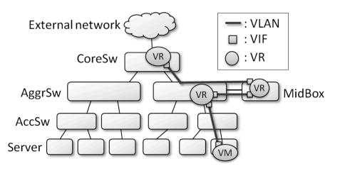
Figure 3.1: Schematic representation of a conventional physical network of datacenter deploying a virtual network for a tenant.
