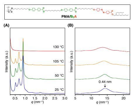
Figure S2 | (A) SAXS and (B) WAXD patterns of a bulk sample of PMA/B<sub>2</sub>A at different temperatures on cooling from its isotropic melt in a glass capillary ( $\phi = 1.5$  mm).
