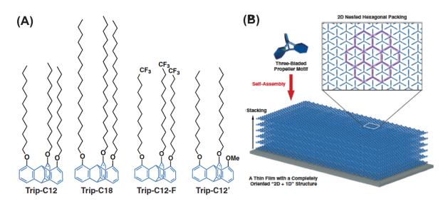
**Figure 12 | The space-filling design to synthesize organic thin films with exceptional long-range structural integrity.** (**A**) Molecular structures of a series of tripodal paraffinic triptycenes. (**B**) Space-filling model with a three-bladed, propeller-shaped motif, capable of forming a "2D hexagonal array + 1D multilayers# by the interpenetration of its propeller parts (nested packing).
