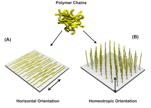
Figure 1 | Schematic illustrations of two different configurations of polymer chains on a substrate. (A) Horizontal orientation of polymer chains lying down on the substrate. (B) Homeotropic orientation of polymer chains vertically standing on the substates.
