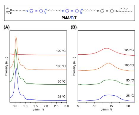
Figure S5 | (A) SAXS and (B) WAXD patterns of a bulk sample of PMA/T<sub>2</sub>T' at different temperatures on cooling from its isotropic melt in a glass capillary ( $\phi = 1.5$  mm).
