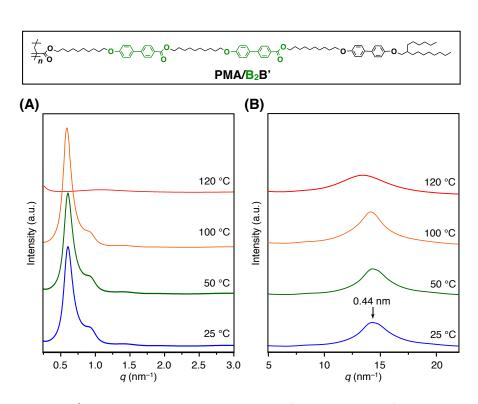
Figure S4 | (A) SAXS and (B) WAXD patterns of a bulk sample of PMA/B<sub>2</sub>B' at different temperatures on cooling from its isotropic melt in a glass capillary ( $\phi$  = 1.5 mm).
