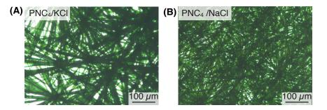
Figure S15 I OM images of PNC₄ sandwiched with two (A) KCl and (B) NaCl plates heating at 180 °C for overnight, respectively.
