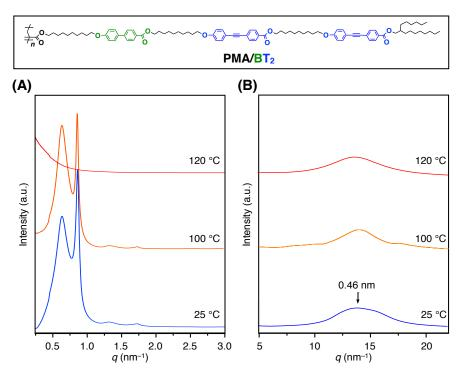
Figure S8 | (A) SAXS and (B) WAXD patterns of a bulk sample of PMA/BT<sub>2</sub> at different temperatures on cooling from its isotropic melt in a glass capillary ( $\phi = 1.5$  mm).
