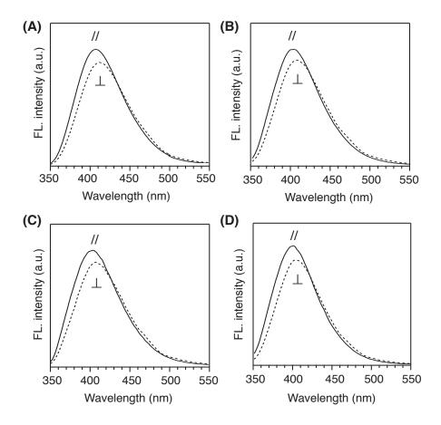
Figure S12 | Polarized emission spectra of (A) PMA/T<sub>3</sub>, (B) PMA/BT<sub>2</sub>, (C) PMA/TBT, and (D) PMA/T<sub>2</sub>B in CHCl<sub>3</sub> (0.1 g/L). The excitation polarizer is parallel (//) and perpendicular ( $\perp$ ) to the emission polarizer, respectively.
