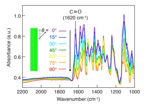
Figure S5 I Polarized IR spectra of the oriented crystalline fibers of Pc4 at azimuthal angle  $\theta$  = 0°, 15°, 30°, 45°, 60°, 75°, and 90°. The azimuthal angle  $\theta$  is defined as zero when the polarizing direction of incident light (blue arrow) is parallel to the long axis of fibrous crystals (green arrow).
