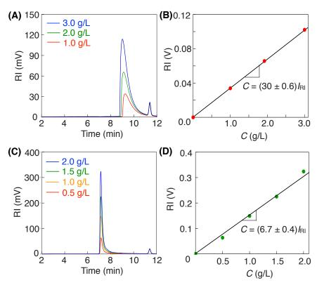
Figure S8 I (A and C) Analytical SEC curves of (A)  $PNC_4$  and (C)  $Pc_4$  in  $CHCl_3$  with different concentrations. (B and D) Standard curves of the intensity of peaks in SEC curves of (B)  $PNC_4$  and (D)  $Pc_4$  versus their concentrations.
