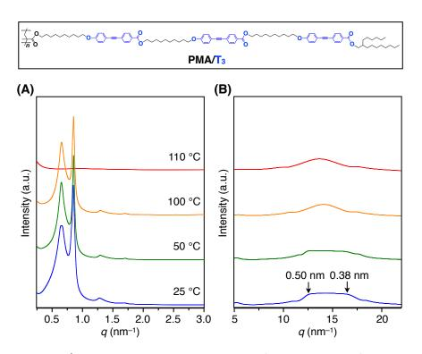
Figure S3 | (A) SAXS and (B) WAXD patterns of a bulk sample of PMA/T<sub>3</sub> at different temperatures on cooling from its isotropic melt in a glass capillary ( $\phi$  = 1.5 mm).
