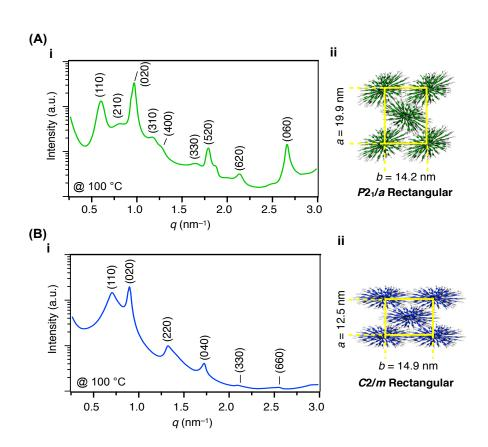
**Figure 5** | **Self-assembled structures of bottlebrush polymers carrying three mesogens in bulk.** 1D SAXS patterns (i) and schematic illustrations of 2D rectangular lattices (ii) of bulk samples of (A) **PMA/B**<sub>3</sub> and (B) **PMA/T**<sub>3</sub> in a glass capillary ( $\phi = 1.5$  mm), measured at 100 °C (mesophase) on cooling from their isotropic melts. Miller indices are given in parentheses.
