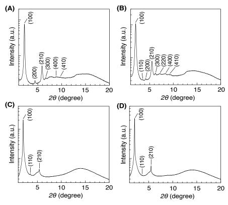
Figure S12 I XRD pattern of powder sample of  $Pc_2$ ,  $Pc_3$ ,  $Pc_5$  and  $Pc_6$  in a glass capillary at 200 °C, 200 °C, 150 °C and 140 °C, respectively. Miller indices in parentheses.
