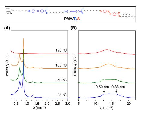
Figure S4 | (A) SAXS and (B) WAXD patterns of a bulk sample of PMA/T<sub>2</sub>A at different temperatures on cooling from its isotropic melt in a glass capillary ( $\phi$  = 1.5 mm).
