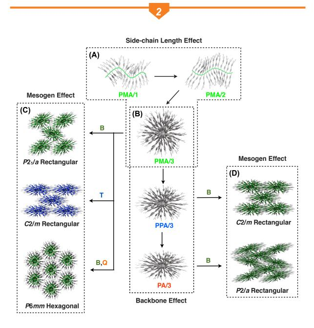
**Figure 11 | Schematic illustrations of 2D rectangular and hexagonal lattices formed by cylindrical brush polymers.** Three main factors, side-chain length (**A**), backbone (**B**), and mesogen (**C** and **D**) affect lattice structures. **PMA**, **PPA**, and **PA** refer to polymethacrylate, polyacrylate and polyphenylacetylene, respectively. **B**, **T**, and **Q** refer to biphenyl, tolan, and quaterthiophene, respectively.
