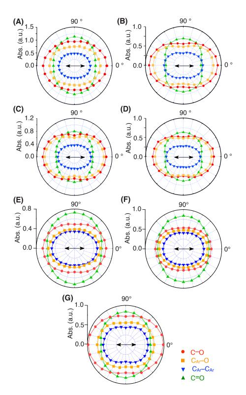
**Figure 9** | Polar plots of the infrared absorption intensities, recorded upon rotation of a polarizer at every 15°, of hot-pressed films of (A) PMA/B<sub>2</sub>A, (B) PMA/BA<sub>2</sub>, (C) PMA/T<sub>2</sub>A, (D) PMA/TA<sub>2</sub>, (E) PMA/T<sub>2</sub>B, (F) PMA/TBT, and (G) PMA/ **BT.** The azimuthal angle is defined as 0° when the polarizing direction of the incident light is parallel to the surface grooves on the Teflon sheets (black arrows).
