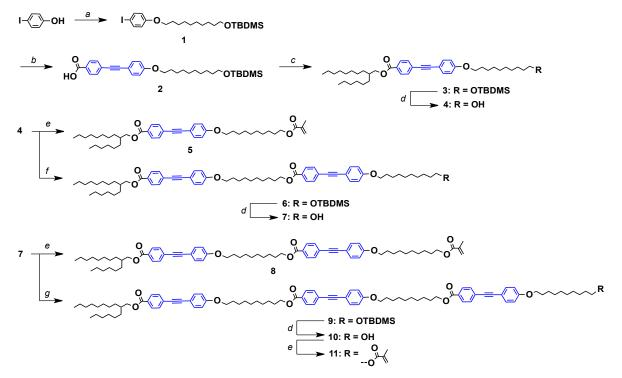
**Scheme S1 I Synthesis of 5, 8 and 11.** *Reagents and conditions:* (a) 10-bromodecyl tert-butyldimethylsilyl ether,  $Cs_2CO_3$ , DMF, 70 °C; (b) 4-ethynylbenzoic acid, Cul, triethylamine, tetrakis(triphenylphosphine) palladium, THF, reflux; (c) 2-hexyl-1-decanol, DPTS, DIPC,  $CH_2CI_2$ , 25 °C; (d) TBAF, THF, 25 °C; (e) methacryloyl chloride, triethylamine,  $CH_2CI_2$ , 25 °C; (f) **2**, DPTS, DIPC,  $CH_2CI_2$ , 25 °C; (g) **2**, DPTS, DIPC,  $CH_2CI_2$ , 40 °C.
