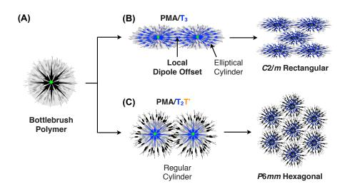
Figure 7 | Schematic illustrations of formation mechanism for 2D rectangular and hexagonal lattices.
