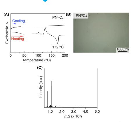
Figure S10 I (A) DSC traces on second heating/cooling cycles (10 °C /min) of PN°C<sub>4</sub>. (B) OM image and (C) MALDI-TOF mass spectra of PN°C<sub>4</sub> after heating at 180 °C in cells for overnight.
