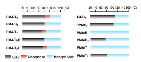
**Figure 4 | Phase transition behavior of polymers.** Thermal properties are characterized by DSC, recorded the second heating/cooling cycles. The scan rate is 5 °C /min.
