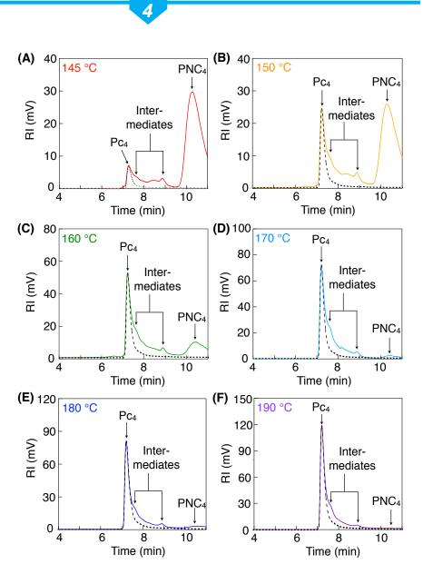
Figure S7 I Analytical SEC curves of the unwashed sample of  $PNC_4$  heating at (a) 145 °C, (b) 150 °C, (c) 160 °C, (d) 170 °C, (e) 180 °C, and (f) 190 °C for 24 hours. Dash line represents the standard curve of the washed fibers of  $Pc_4$ .
