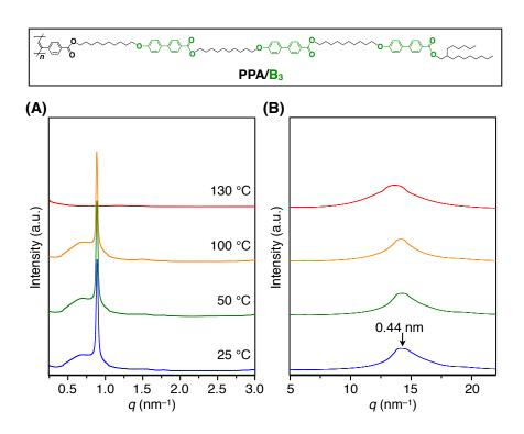
Figure S7 | (A) SAXS and (B) WAXD patterns of a bulk sample of PPA/B<sub>3</sub> at different temperatures on cooling from its isotropic melt in a glass capillary ( $\phi$  = 1.5 mm).
