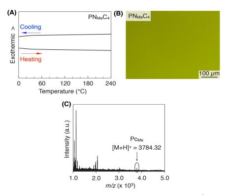
Figure S9 I (A) DSC traces on second heating/cooling cycles (10 °C /min) of PN<sub>Me</sub>C<sub>4</sub>. (B) OM image and (C) MALDI-TOF mass spectra of PN<sub>Me</sub>C<sub>4</sub> after heating at 180 °C in cells for overnight.
