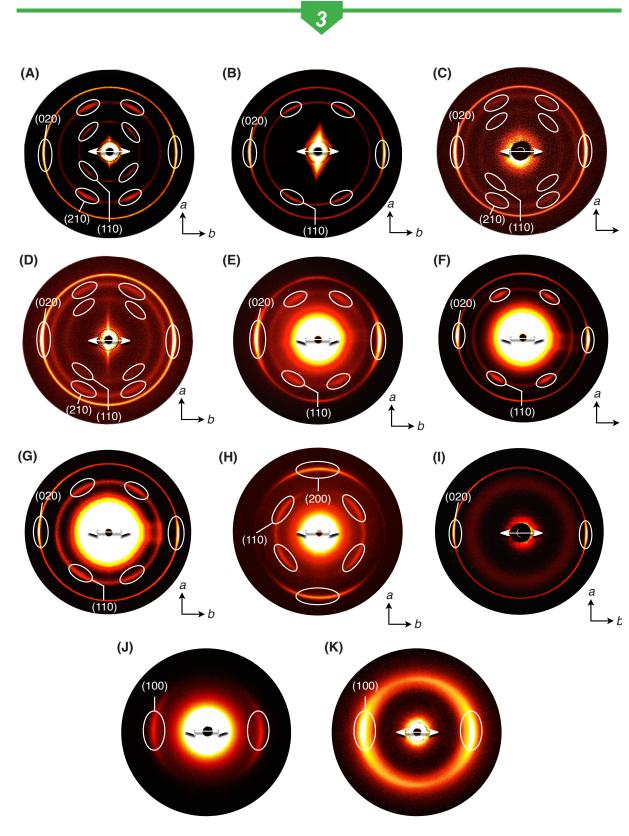
Figure 6 I Through-view 2D SAXS images at 25 °C of hot-pressed films of (A) PMA/B<sub>2</sub>A, (B) PMA/BA<sub>2</sub>, (C) PMA/T<sub>2</sub>A, (D) PMA/TA<sub>2</sub>, (E) PMA/T<sub>2</sub>B, (F) PMA/TBT, (G) PMA/BT<sub>2</sub>, (H) PA/B<sub>3</sub>, (I) PPA/B<sub>3</sub>, (J) MA/B<sub>3</sub>, and (K) MA/T<sub>3</sub> prapered with parallel arranged Teflon sheets. White arrows denote the directions of grooves on the Teflon sheets.
