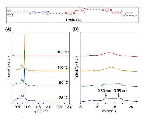
Figure S5 | (A) SAXS and (B) WAXD patterns of a bulk sample of PMA/TA<sub>2</sub> at different temperatures on cooling from its isotropic melt in a glass capillary ( $\phi$  = 1.5 mm).
