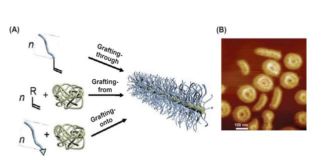
**Figure 7 | Synthetic strategies and morphologies of brush polymers. (A)** Schematic illustration of three main synthetic strategies: grafting through (polymerization of macromonomers), grafting onto (polymerization of polymeric side chains from backbone), and grafting from (pasting polymeric side chains to backbone).<sup>54</sup> (**B**) AFM images of bottlebrush polymers and its ring structure, prepared by spin coating of a dilute solution.<sup>56</sup>
