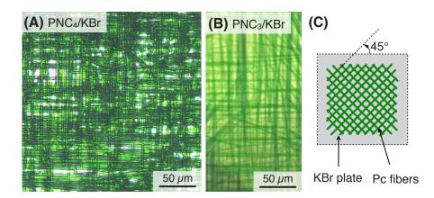
Figure 6 | 2D orthogonal orientation of Pc crystalline fibers on KBr plates. (A, B) OM images of Pc crystalline fibers after heating (A)  $PNC_4$  and (B)  $PNC_3$  sandwiched with two KBr plates at 180 °C for overnight, respectively. (C) Schemtic illustration of 2D orthogonal orientation of crystalline fibers on KBr plates.
