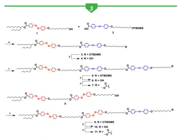
**Scheme S11 Synthesis of 7 and 11.** *Reagents and conditions:* (a) **2**, DPTS, DIPC,  $CH_2Cl_2$ , 25 °C; (b) TBAF, THF, 25 °C; (c) **2**, DPTS, DIPC,  $CH_2Cl_2$ , 40 °C; (d) methacryloyl chloride, triethylamine,  $CH_2Cl_2$ , 25 °C.
