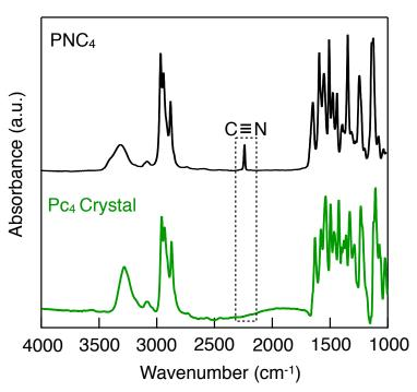
Figure S3 I IR spectra of PNC<sub>4</sub> (black line) and crystalline fibers of Pc<sub>4</sub> (green line) on KBr substrates.
