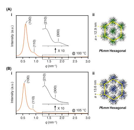
**Figure 6** | **Self-assembled structures of brush polymers containing a apolar mesogen in bulk.** 1D SAXS patterns (i) and schematic illustrations of 2D lattices (ii) of bulk samples of (A) PMA/B<sub>2</sub>B' and (B) PMA/T<sub>2</sub>T' in a glass capillary ( $\phi$  = 1.5 mm), measured at 100 °C (mesophase) on cooling from their isotropic melts. Miller indices are given in parentheses.
