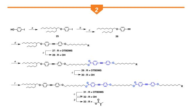
**Scheme S3 I Synthesis of 33.** *Reagents and conditions:* (a) 1-bromo-2-hexyldecane,  $Cs_2CO_3$ , DMF, 70 °C; (b) Trimethylsilylacetylene, Cul, triethylamine, tetrakis(triphenylphosphine)palladium, THF, reflux; (c) TBAF, THF, 25 °C; (d) **1**, Cul, triethylamine, tetrakis(triphenylphosphine)palladium, THF, reflux; (e) **2**, DPTS, DIPC,  $CH_2CI_2$ , 25 °C; (f) **2**, DPTS, DIPC,  $CH_2CI_2$ , 40 °C; (g) methacryloyl chloride, triethylamine,  $CH_2CI_2$ , 25 °C.
