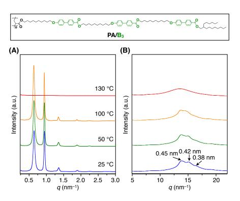
Figure S6 | (A) SAXS and (B) WAXD patterns of a bulk sample of PA/B<sub>3</sub> at different temperatures on cooling from its isotropic melt in a glass capillary ( $\phi$  = 1.5 mm).
