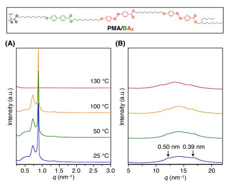
Figure S3 | (A) SAXS and (B) WAXD patterns of a bulk sample of PMA/BA<sub>2</sub> at different temperatures on cooling from its isotropic melt in a glass capillary ( $\phi = 1.5$  mm).
