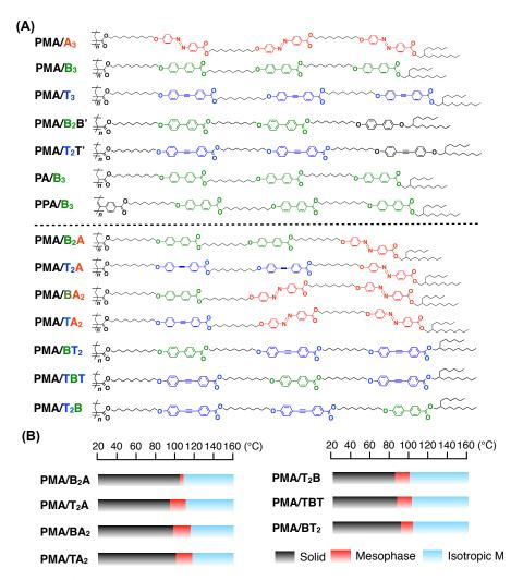
**Figure 3** | (A) Molecular formulae of existing (up) and newly synthesized (down) brush polymers. (B) Phase transition behavior of newly synthesized (down) brush polymers. Thermal properties are characterized by DSC, recorded the second heating/cooling cycles. The scan rate is 5 °C /min. Black arrows denote the shifted direction of phase transition temperatures.
