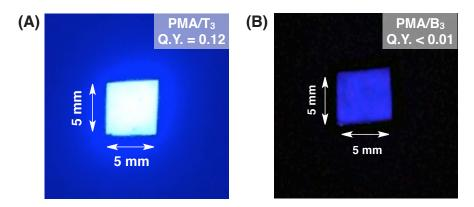
Figure S11 | Photographs of hot-pressed films (5 mm × 5 mm) of (A) PMA/ $T_3$  and (B) PMA/ $B_3$  irradiated by UV light (365 nm). The fluorescence quantum yield of hot-pressed PMA/ $T_3$  film was 0.12, while that of hot-pressed PMA/ $B_3$  flim was only less than 0.01.
