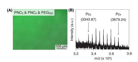
Figure S13 I (A) OM image and (B) MALDI-TOF mass spectra of a mixture of  $PNC_3$ ,  $PNC_4$  (mole ratio = 1/1) and  $PEG_{500}$  (10%wt) heating at 180 °C for overnight.
