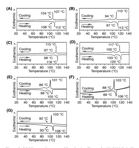
Figure S1 | DSC traces in a second heating/cooling cycle. (A) PMA/B<sub>2</sub>A, (B) PMA/BA<sub>2</sub>, (C) PMA/T<sub>2</sub>A, (D) PMA/TA<sub>2</sub>, (E) PMA/T<sub>2</sub>B, (F) PMA/TBT, and (G) PMA/BT<sub>2</sub>. Scan rate is 5 °C min<sup>-1</sup>.
