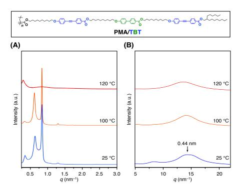
Figure S7 | (A) SAXS and (B) WAXD patterns of a bulk sample of PMA/TBT at different temperatures on cooling from its isotropic melt in a glass capillary ( $\phi = 1.5$  mm).
