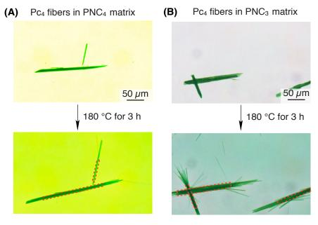
**Figure S14 I OM images of the Pc**<sub>4</sub> **fibrous seeds in (A) PNC**<sub>4</sub> **and (B) PNC**<sub>3</sub> **matrix heating at 180 °C for 3 hours.** The red frames represent the initial shape of **Pc**<sub>4</sub> fibrous seeds.
