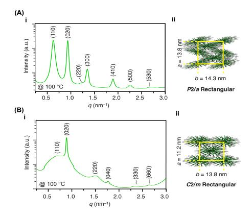
**Figure 10 | Self-assembled structures of brush polymers with different backbones in bulk.** 1D SAXS patterns (i) and schematic illustrations of 2D rectangular lattices (ii) of bulk samples of (A) PA/B<sub>3</sub> and (B) PPA/B<sub>3</sub> in a glass capillary ( $\phi = 1.5$  mm), measured at 100 °C on cooling from their isotropic melts. Miller indices are given in parentheses.
