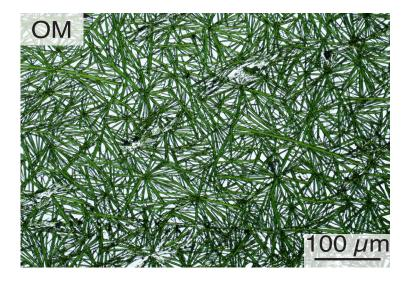
Figure S2 I OM images of the crystalline fibers of  $Pc_4$  washed by methanol at 25 °C.
