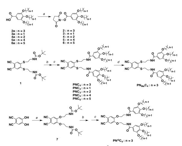
Scheme S1 I Synthesis of PNC<sub>n</sub> (n = 2 ~ 6), PN<sub>Me</sub>C<sub>4</sub> and PN<sup>o</sup>C<sub>4</sub>. *Reagents and conditions:* (a) NHS, DCC, 1,4-dioxane, 25 °C; (b) TFA, CH<sub>2</sub>Cl<sub>2</sub>, 25 °C; (c) 2 ~ 6, Et<sub>3</sub>N, CH<sub>2</sub>Cl<sub>2</sub>, 25 °C; (d) NaH, MeI, THF, 25 °C; (e) t-butyl 2-bromoethylcarbamate , K<sub>2</sub>CO<sub>3</sub>, DMF, 70 °C.
