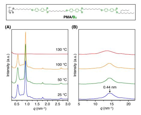
Figure S2 | (A) SAXS and (B) WAXD patterns of a bulk sample of PMA/B<sub>3</sub> at different temperatures on cooling from its isotropic melt in a glass capillary ( $\phi = 1.5$  mm).
