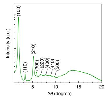
**Figure S4 I XRD pattern of powder sample of Pc**<sub>4</sub> **in a glass capillary at 180 °C.** Miller indices in parentheses.
