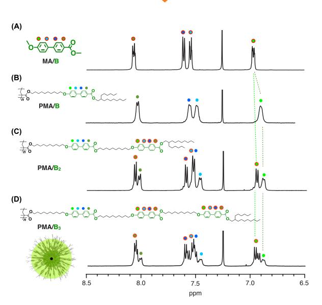
**Figure 9** | <sup>1</sup>**H** NMR spectra of biphenyl units of monomer and polymers in CDCl<sub>3</sub> solution. (A) MA/B, (B) PMA/B, (C) PMA/B<sub>2</sub>, and (D) PMA/B<sub>3</sub> are selected from 6.5 to 8.5 ppm. In a cylindrical shape, side chains of PMA/B<sub>3</sub> extend isotropically without entanglement.
