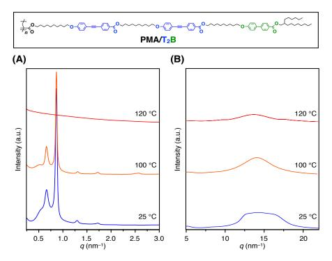
Figure S6 | (A) SAXS and (B) WAXD patterns of a bulk sample of PMA/T<sub>2</sub>B at different temperatures on cooling from its isotropic melt in a glass capillary ( $\phi = 1.5$  mm).
