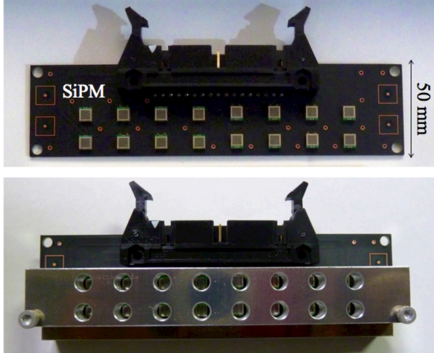
Figure 5-6: Printed circuit board for SiPM mount and fiber connection: (upper) printed circuit board after SiPM implementation; (lower) circuit board with the aluminum support for fiber bundle connection to the SiPM.
