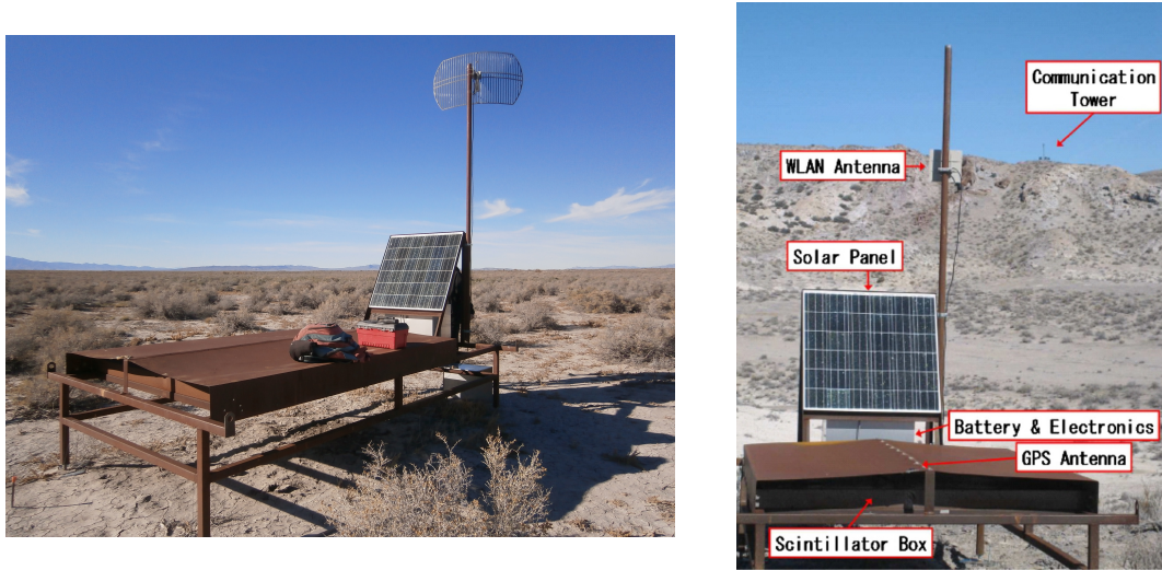
Figure 2.3: The TA SD deployed in the TA site. (left) The overview of the detector. (right) The explanation of each part [58]. The SK communication tower is seen behind on the hill.
