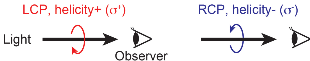
FIGURE 2.1: Definition of circular polarization and the helicity.
