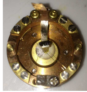
(b) The capacitive transducer using in magnetization measurements of CuPzN (Chapter 3).
