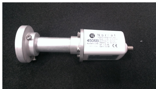
Figure 2.9: The block converter (Norsat 4506B) which was used as receiver in the experiment by Horie et al.
