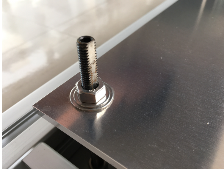
Figure 3.7: Photograph for the corner of mirror. It is fixed using a screw and washers and nuts.
