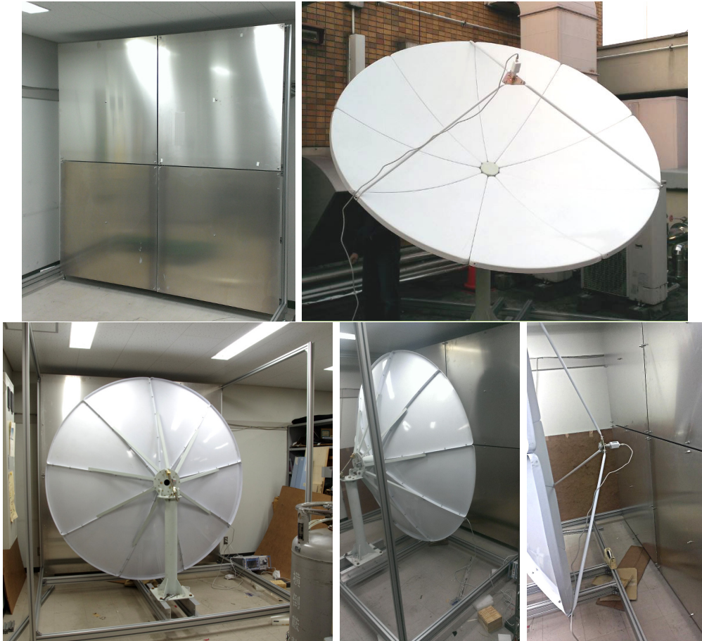
Figure 2.8: The set up of the HPCDM search experiment by Horie et al. A plane mirror (upper left) was made of 4 pieces aluminum plate. A parabola antenna (upper right) is used for collecting converted plane wave from the mirror. They are combined in HPCDM search measurement (bottom).
