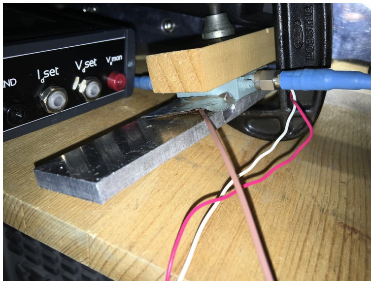
Figure 3.19: The room temperature amplifier is clamped to an aluminum plate as a heat radiator. A temperature sensor is attached here with an adhesive tape.
