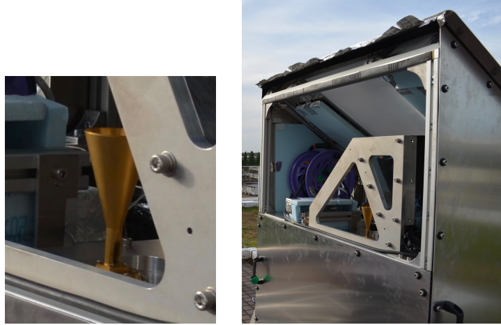
Figure 3.11: The housing of the receiver. The horn antenna sees sky through a microwave-transparent window. This housing holds the cryostat (Fig. 3.10) and other facilities, such as spectrum analyzers, room temperature amplifiers, computers, an uninterruptible power supply (UPS).
