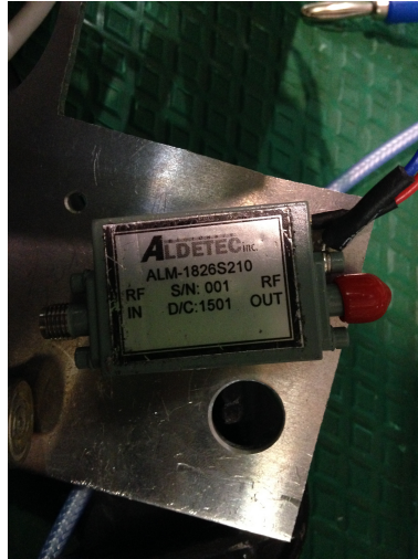
Figure 3.16: Room temperature amplifier, ALM-1826S210 (Aldetec).
