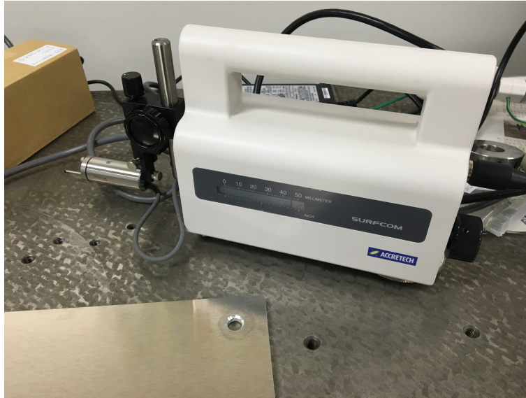
Figure 6.28: The surface roughness measurement machine we used
