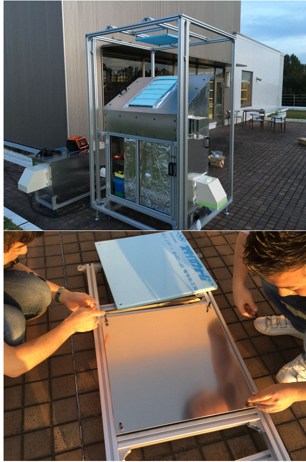
Figure 3.6: The aluminum mirror is hinged above the receiver. We replace the mirror to styrofoam plate for antenna area calibration described in Section 5.2. Plates have four holes at their corners. We used screws and nuts to set them with alignment for their direction to the line of sight of the receiver.
