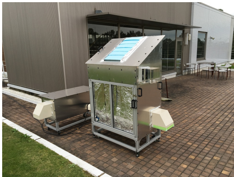
Figure 3.12: KUMODES (the receiver). The housing protects facilities inside from rains and winds.
