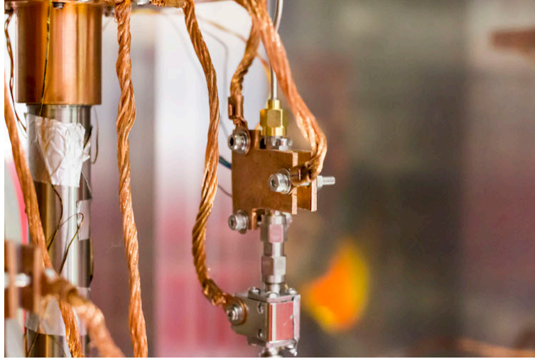
Figure 3.15: Cryogenic Low Noise Amplifier, LNF-LNC15.29A (LOW NOISE FACTORY). This is set in the cryostat. Photo Courtesy of KEK IPNS/Shota Takahashi.
