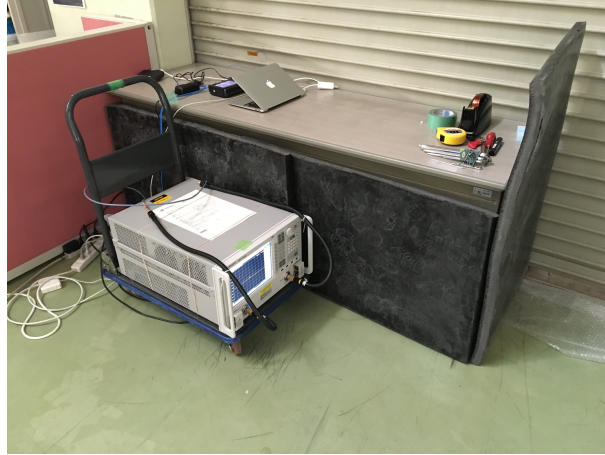
Figure 5.19: Picture of the setup described in Fig. 5.18. The front instrument is VNA used as generate a monotone signal. Spectrum analyzer is under the desk, and surrounded by boards. The shutter in the back was opened to lower ambient temperature around the spectrum analyzer.
