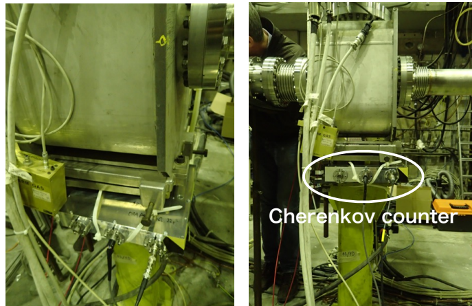
FIGURE 2.16: Photos of the Cherenkov counter. It was placed under GEM47 which functioned as a beam dump.
