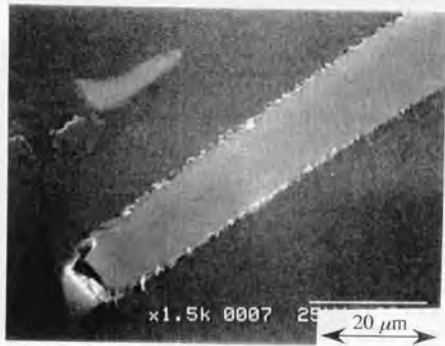
Figure 3-25. Microvoid occurring at the interface separating the fibre tip from the matrix and interfacial microfailure along the fibre sides, which were obtained under about 85% of failure load.
