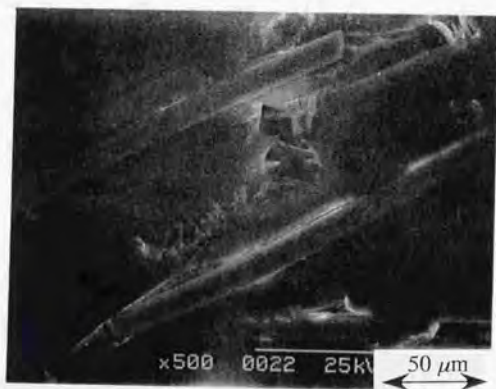
Figure 3-27. Crack opening occurring in the large plastic deformation band of the matrix, which was obtained under about 95% of failure load.
