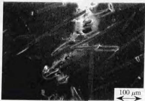
Figure 3-28. Fast crack propagation of the matrix with fibre pull-out, which was obtained under load just before failure.
