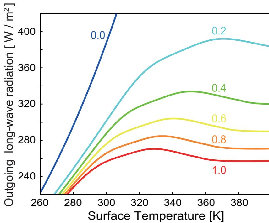
Figure 3.10. 1-D radiation limit with various values of the relative humidity, obtained by use of the radiation code in AGCM 5.4g.
