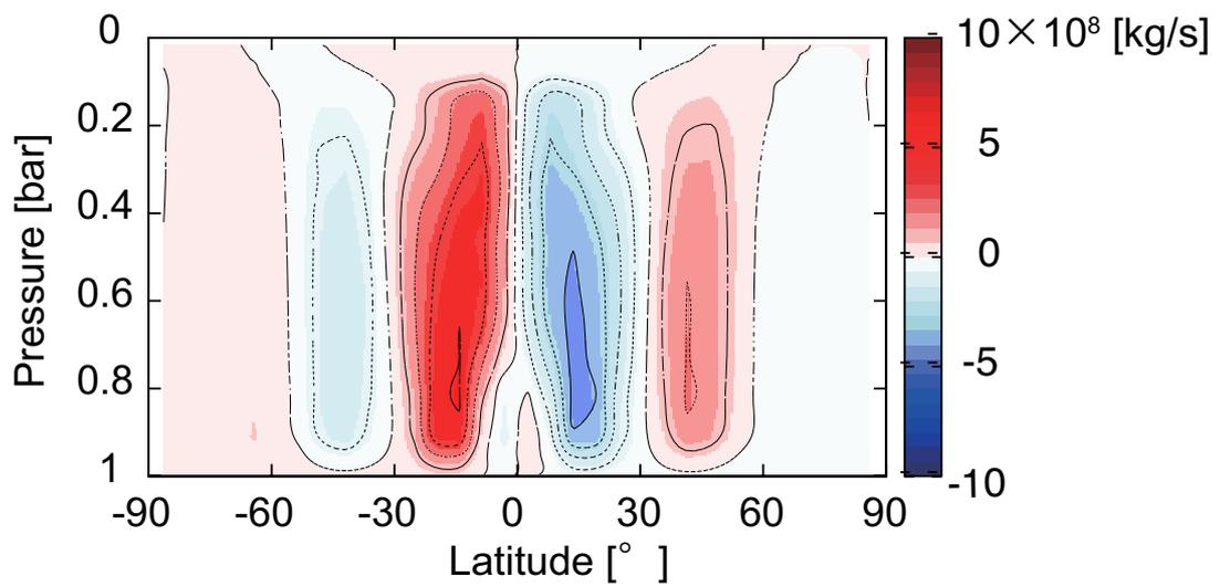
Figure 3.7. The mass stream function in the case of the water flow limit =  $19.3^\circ$ . Negative values represent the mass stream of right-hand circular and, on the other hand, positive values represent that of left-hand circular.
