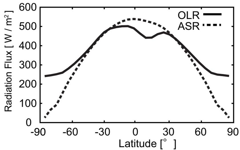
Figure 3.5. The absorbed shortwave radiation (ASR, dashed line) and the outgoing long-wave radiation (OLR, solid line) in the case of the water flow limit =  $69.2^\circ$ . Note that, in lower latitudes, a very large OLR is found to be emitted.
