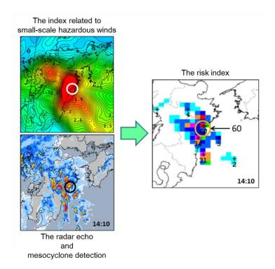
**Fig. 1-5.** A schematic image of the decision process for the risk index of small-scale hazardous winds adopted in JMA. (Adapted from the image open to the public in the JMA's website: http://www.jma.go.jp/jma/kishou/know/toppuu/tornado2-3.html)
