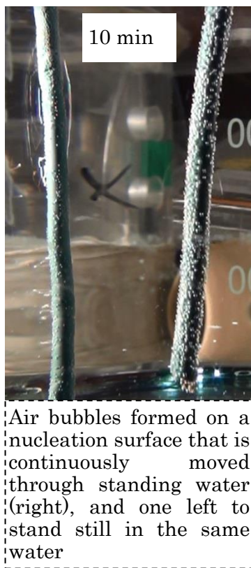
Figure 5-9: Water movement acts to bring air-rich water to the interface while at the same time take away de-aired water away from the interface. It is either water movement over the bubble or bubble movement through the water.
