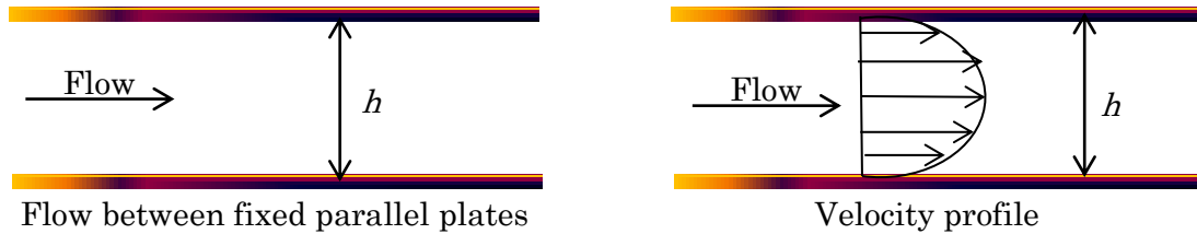
Figure 2-10: Velocity profile for flow of an incompressible liquid between two fixed parallel plates, assuming laminar flow conditions.
