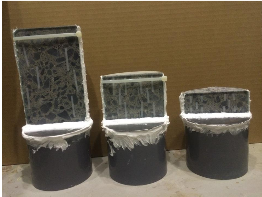
Concrete – Glass specimens of different sizes to check effect of water flow
