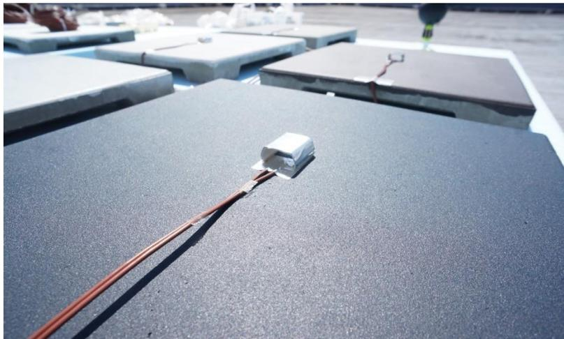
Figure 6-20 A custom made plastic caps with an aluminium foil finishing are placed to protect the thermocouple probes from the direct sunlight throughout the day.
