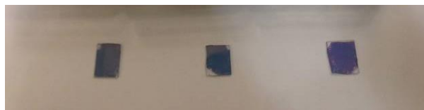
Figure 4-3: Photo of GNIs on Sapphire substrate annealed at 500°C (left), 700°C (center), 900°C (right). Samples show blue color due to plasmonic absorption.
