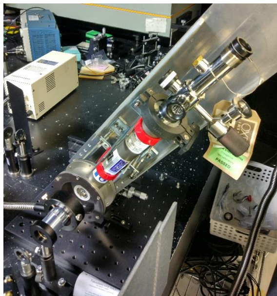
Figure 2-10: Picture of Cryostat (Oxford Instruments, MicrostatHe2) for the TDTR system. The cryostat chamber is cooled by liquid helium.
