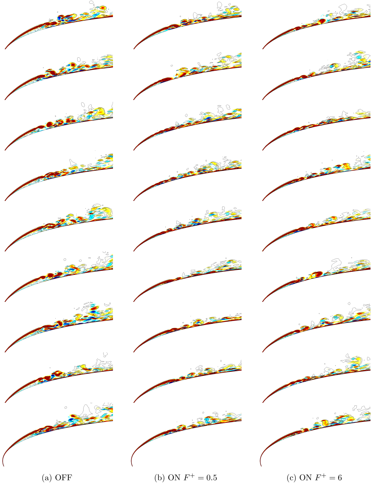
Figure 5.19: Side-view for instantaneous flowfield around the leading edge shear layer in the phase of 65^\circ . The black line contour depicts the second invariant of the velocity gradient tensor, and color contour depicts the spanwise vorticity. Time lapses from top to bottom with time increment of tu_\infty/c = 0.065 .
