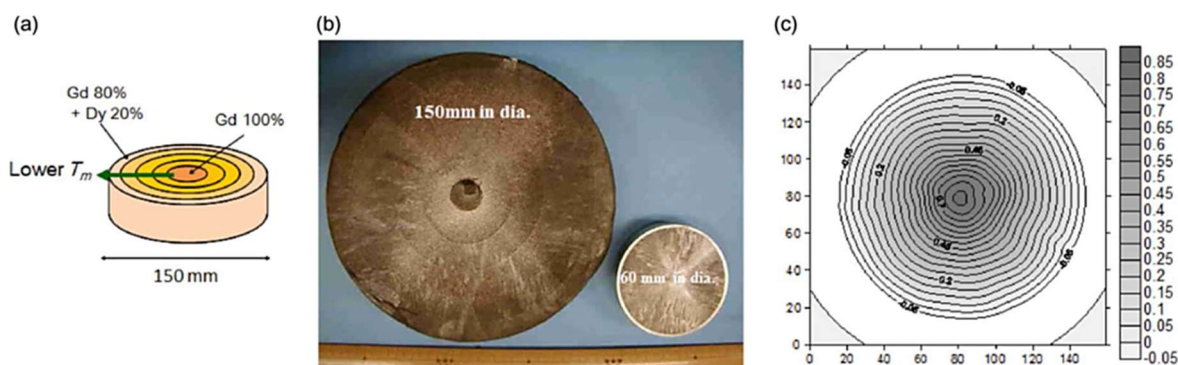
Fig. 8-10 Schematic illustration of RE compositional gradient method (a), top view of Gd-based QMG (150 mm \phi ) of GdBCO with a compositional gradient of Dy (b) and distribution of trapped field at 87 K (in liquid Ar) (c). 109
