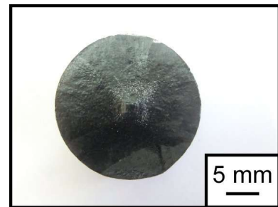
Fig. 7-26 Top views of failed Ag-added (Y, Er)BCO melt-textured bulks (~20 mm \phi ).
