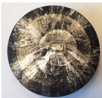
Fig. 8-8 Top view of YBCO bulk prepared from precursor pellet with graded change of Y-211 concentration. 204
