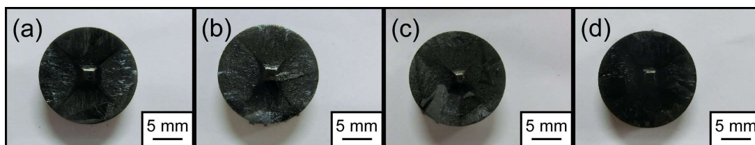
Fig. 4-17 Top views of (Gd,Gd)BCO (a), (Gd,Dy)BCO (b), (Gd,Y)BCO (c) and (Dy,Gd)BCO (d).
