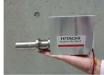
Fig. 1-48 Structure and photo image of the trial palm-sized HTS bulk magnet. 130
