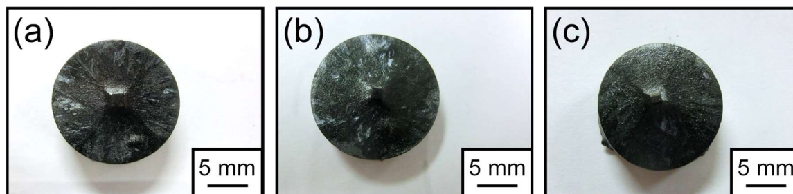
Fig. 4-30 Top views of (Ho,Ho)BCO (a), (Ho,Er)BCO (b), (Er,Er)BCO (c).
