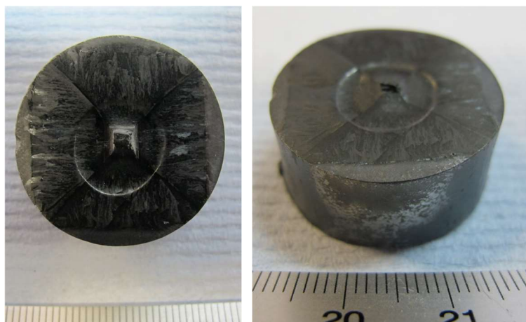
Fig. 8-14 Photo images of graded (Y,Dy)BCO melt-textured bulk.
