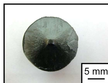
Fig. 8-20 Top view of Ag-added (Gd,Gd)BCO melt-textured bulk with 2 wt% BaO 2 .
