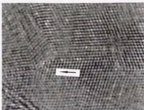
Figure 3.14: HRTEM of the multiply-twinned particles in c -BN film.
