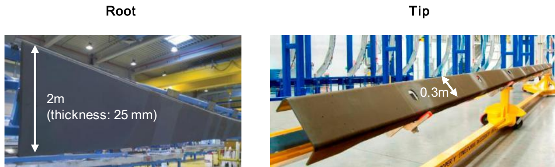
Fig. 6.2: Different size and shape of aircraft wing spar along longitudinal direction [122,128].
