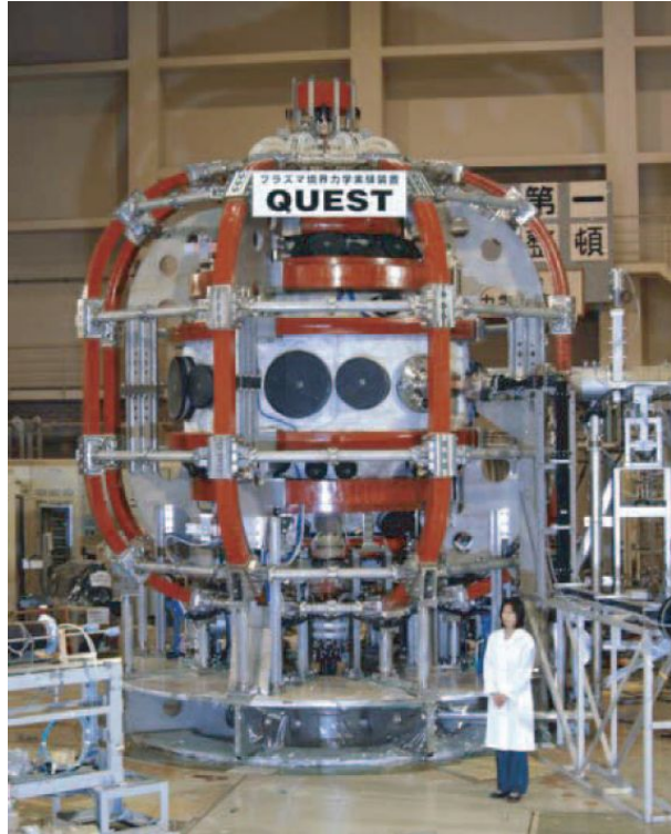
Fig. 5.1: Photograph of the vacuum vessel and TF and PF coils of QUEST [21].
