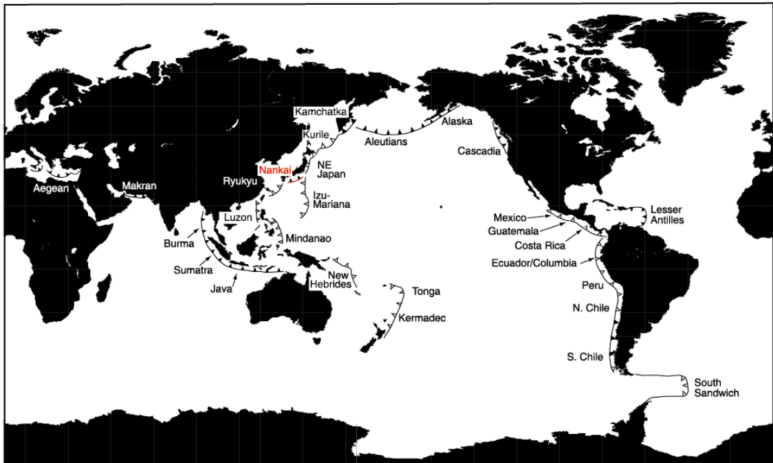
Figure 1.1 Map showing the distribution of subduction zones of the world. Accretionary margins are shown with solid bars on the plate boundary, while open bars mark erosive margins. Modified from Clift et al. [2004].
