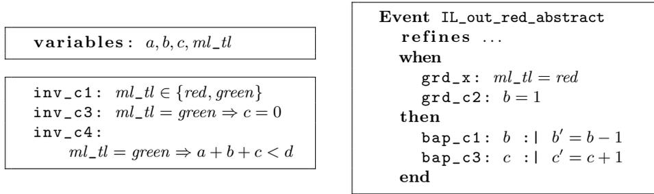
Figure 3.2: Part of abstract machine (about  $\{a, b, c, ml\_tl\}$ ) of traffic example
