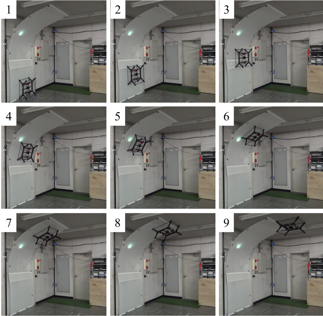
図 5.23: Wall trace locomotion: We took the challenge of movement touching a wall with a curved shape.
