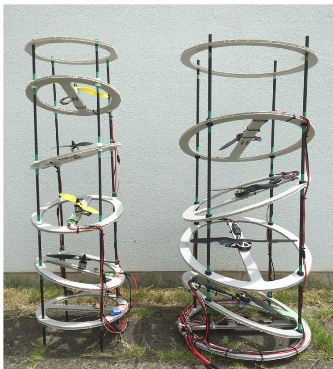
図 3.89: ASAGAO: Cylindrical coaxial four propellers multi rotor flying robot
