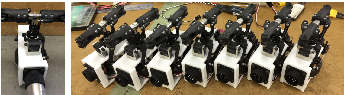
図 2.19: Removable variable pitch propeller module (Developed in 2014)
