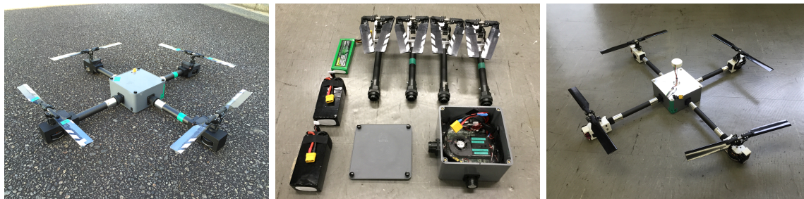
図 3.52: Removable arm variable pitch propeller quad rotor flying robot (Developed in 2014)
