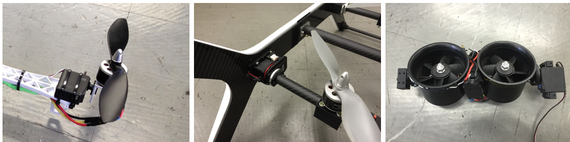
図 2.27: Variable thrust propeller module (Developed in 2015-2016)
