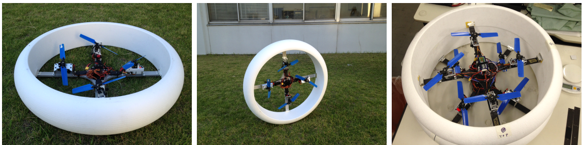
図 3.107: MUWA2: Tilted thrust MUWA (Developed in 2013)
