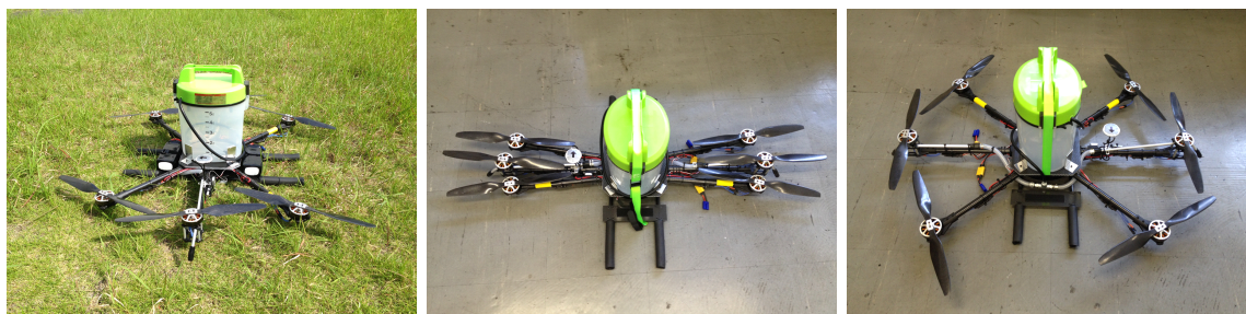
図 3.49: Pesticide spraying multi rotor flying robot for agriculture (Developed in 2013)
