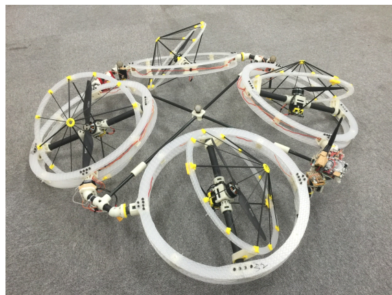
図 3.113: Gimbal propeller module multi rotor (Developed in 2015)
