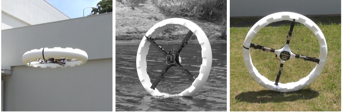
図 4.2: (1)Flying (2)Stand and Floating (3)Stand and Rolling
