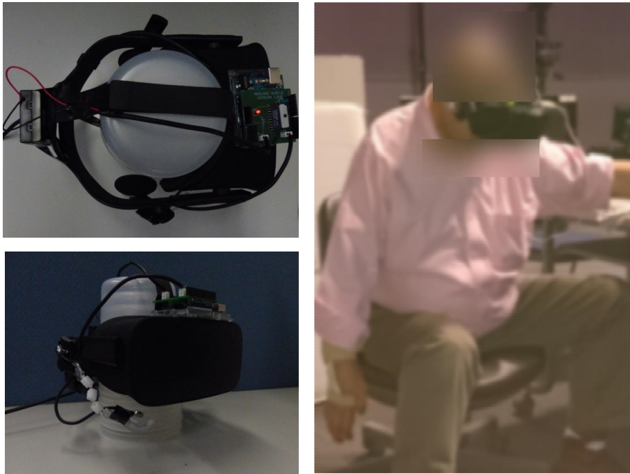
Fig. 8.1: Portable home-use VR system for long-term VR rehabilitation
