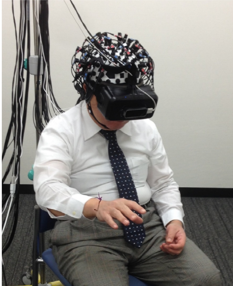
Fig. 5.1: Attachment of both NIRS and VR rehabilitation system
