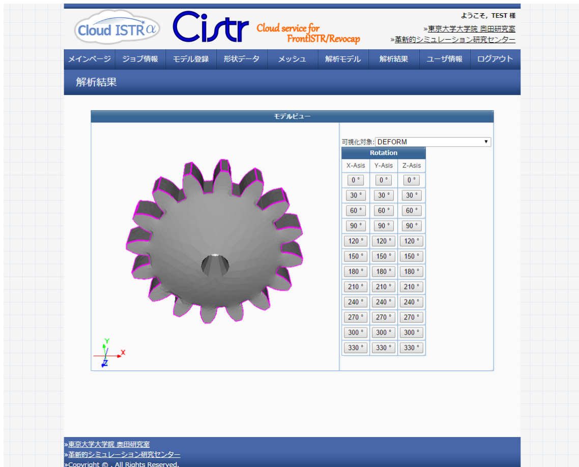
Fig 8.13: Deformed image of gear model FEM result
