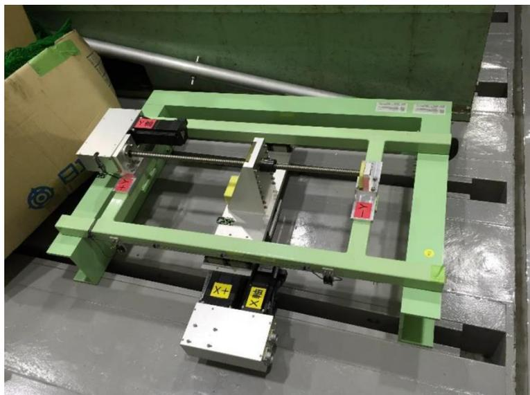
Figure 2-6 Forced vibration device
