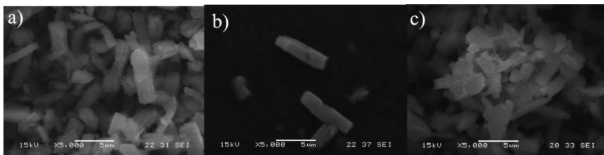
Figure 4-23 Scanning electron microscope of H-ZSM-5(1500) a) before reaction b) after operating 6 hours in supercritical water at temperature 400^\circ\text{C} with pure water and c) with Si Al solution
