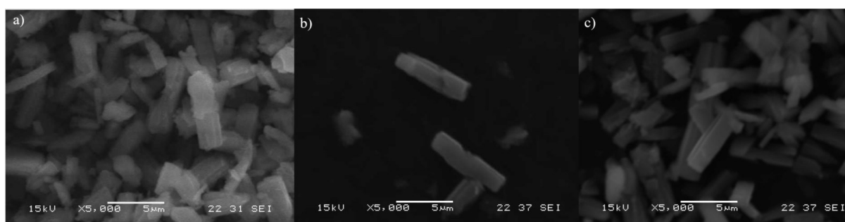
Figure 4-14 Scanning electron microscope of H-ZSM-5(1500) a) fresh zeolite before operating in supercritical water, and after at pressure b) 24.1 MPa c) 26.9 MPa.
