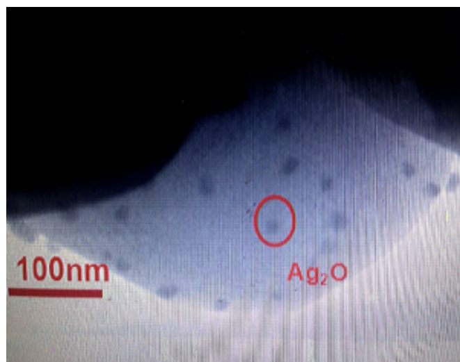
Fig.4-2 TEM image of Ag 2 O/ TiO 2 ;673 K, 35 MPa, 0.03 mol -1 .
