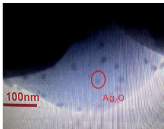
Fig.4-5 TEM image of Ag 2 O/ TiO 2 ;673 K, 35 MPa, 0.03 mol -1 CH 3 COOAg.
