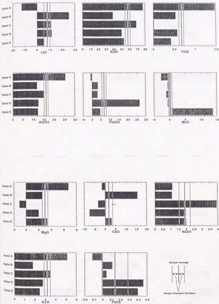
Figure 15: Composition scores of factors calculated by Q-mode factor analysis for all analyzed samples using all elements with varimax rotation.
