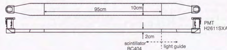
Figure 2.23: Time-of-flight counter of BESS '95 instrument.
