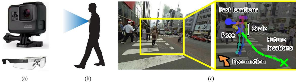
**Figure 1.1.: Future person localization.** (a) An example of a wearable camera (upper: GoPro HERO, lower: Google glass.) (b) Camera configuration used in this work. A wearable camera is mounted on the wearer’s chest. (c) Given a first-person video of a certain target person, our network predicts where the target person will be located in the future frames based on the poses and scales of the person as well as the ego-motions of the camera wearer.
