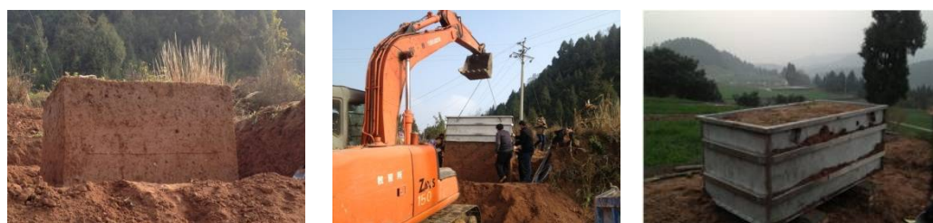
Figure 2-2 Collection of the undisturbed soil box from an upland cropland field
