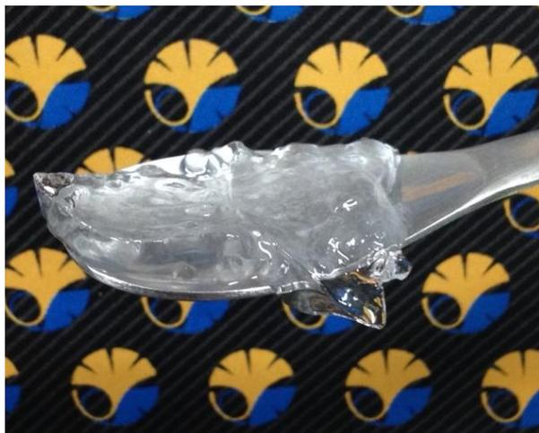
**Figure 2-8** Gel-like precipitates were formed when the 1% w/v LiCl/DMAc A-chitin solution was diluted to 0.5% w/v LiCl/DMAc.
