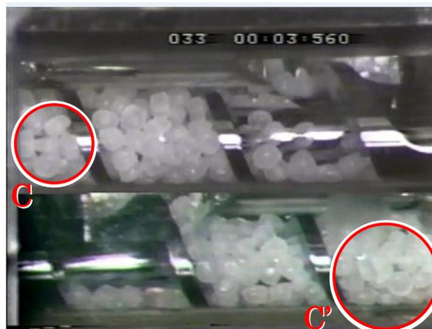
(3) Screw rotation rate 30 rpm, starvation ratio 6 %
