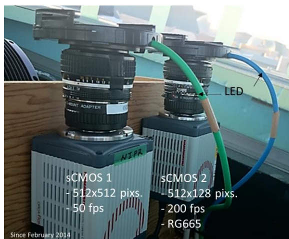
Figure 2.9: Two sCMOS cameras equipped with the identical NIKKOR 50 mm/F 1.2 lens and the LED light.
