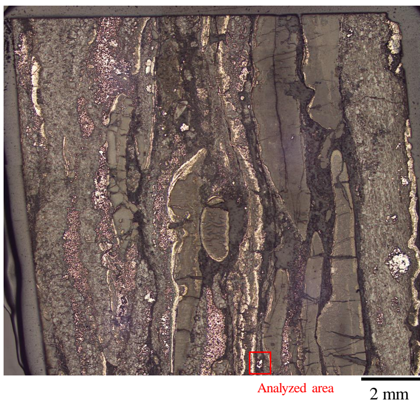
Fig. III-4 Optical micrograph of black shale sample.
