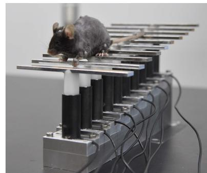
Fig.6 Outline of the stairs for mouse force measurement
