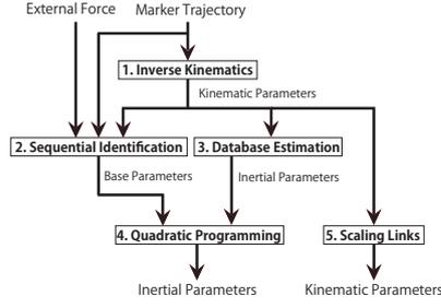
Fig.2 Outline of the proposed method to identify kinematic and inertial parameters
