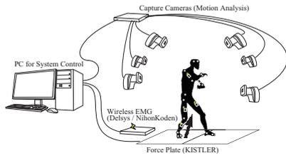
Fig.3 Motion capture system
