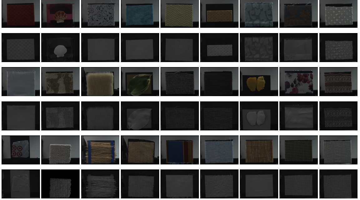
Figure 4.6: Selected RGB-NIR image pairs that satisfy the property that surfaces of captured objects have diffused reflectance. From left to right and top to bottom, the materials are (same name used in NISAR dataset): artificialLeather-polyester-suede, artificialShell, blackNwhite-jacquardPolyester, blue-quilterFlannel, chevronYellow-poly-cotton, cracker, floralJacquard-polyester, flowerPattern-thickCotton, ivoryDot-polyester, jacquardPoly-spandex, jute, lamb-swool, leaf-twoColor, olefin_polyester-cotton, olefin-cotton-polyester, orange, peachPrints-polyester, pinkChiffon, plasticBag1, pureColorDyedBCFNylon-white, straw, straw2, tableCloth-cotton, tealStich-thinCotton, woodTexture-quilterFlannel, woolScarf and yellow-seersuckerCotton.
