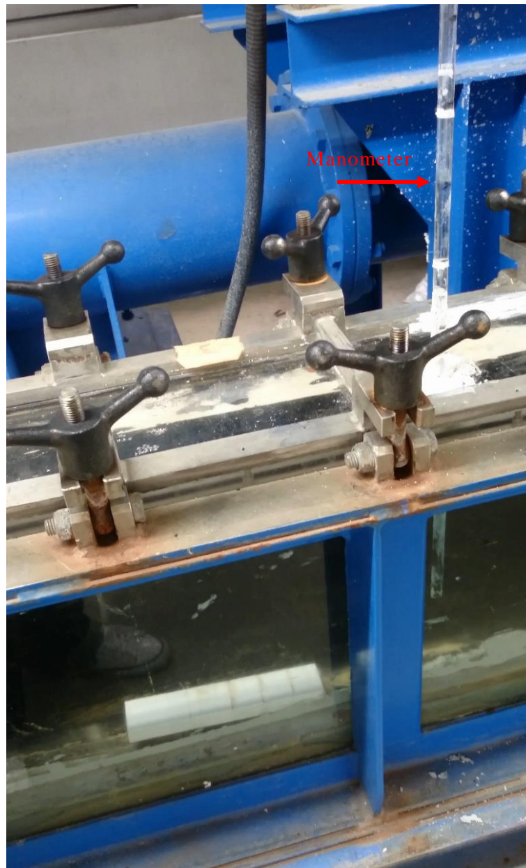
Figure 14 A manometer placed on the lid of OFT
