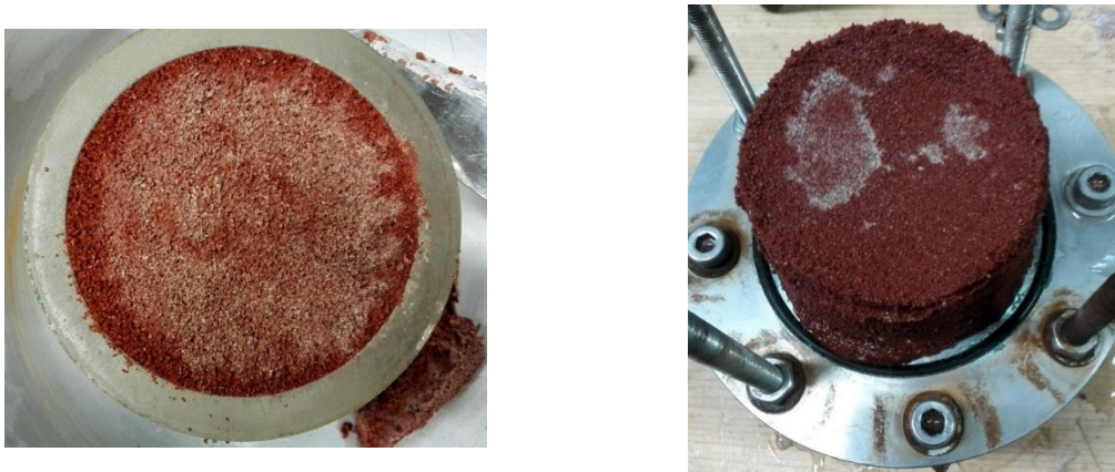
Figure 4-5 Specimens after erosion: Dense specimen (left) Loose specimen (right)
