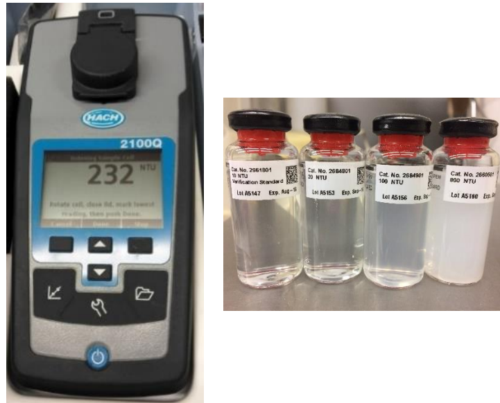
Figure 3-12 Turbidimeter HACH 2100Q and samples used for calibration
