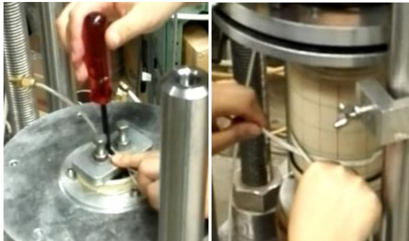
Figure 3-48 Cap for the inner hollow and diameter measurement
