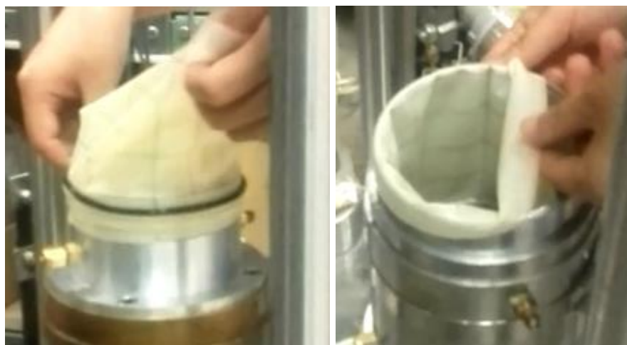
Figure 3-44 Outer membrane and outer mold
