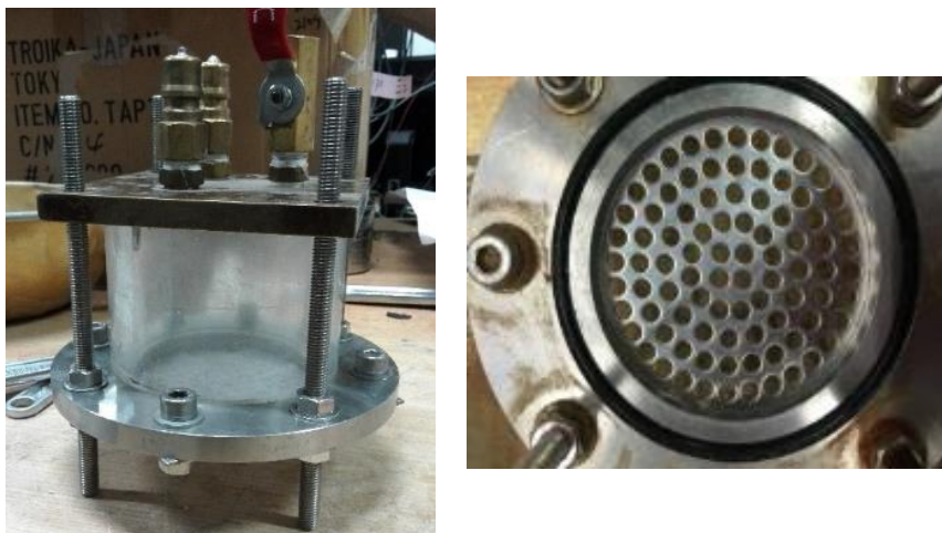
Figure 3-11 Soil chamber with holes on the bottom plate
