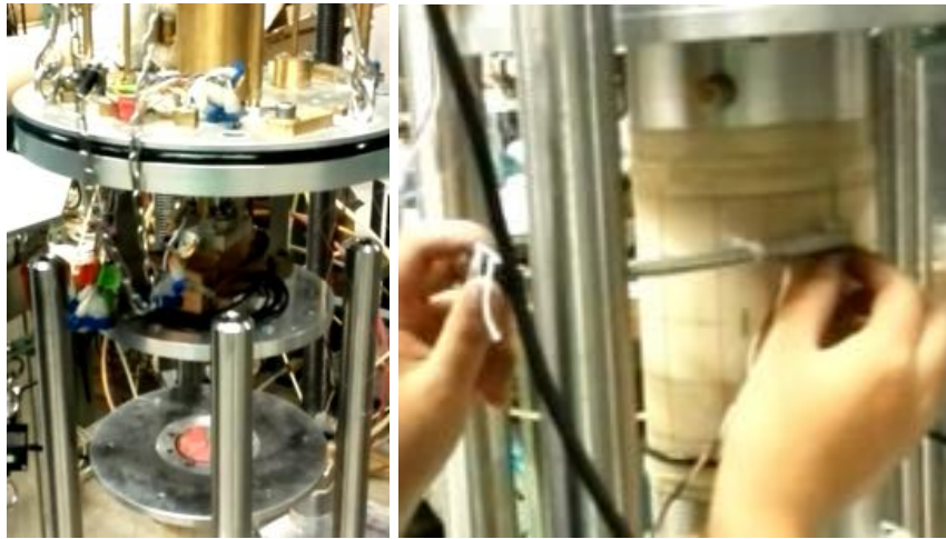
Figure 3-49 Placement of the load cell cap and clip gauges
