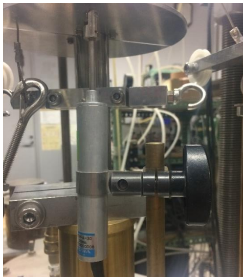
Figure 3-26 Linear Variable Differential Transducer (LVDT)
