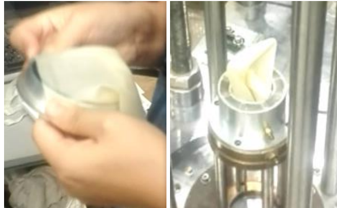
Figure 3-43 Inner membrane and base pedestal
