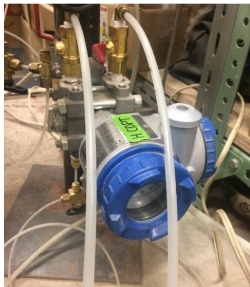
Figure 3-22 High Capacity Differential Pressure Transducer HCDPT
